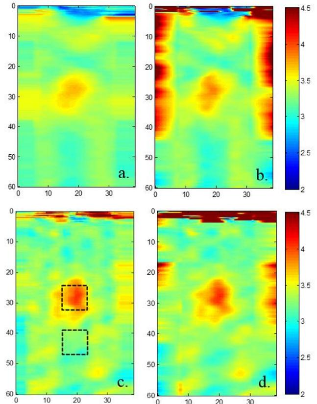
Fig. 5. SWS images (m/s) of an inclusion phantom at (a, b) 280 Hz and (c, d) 500 Hz vibration frequency. Left side: WAVE. Right side: PD. Measurement are shown in mm. Squares windows of 8mm were used for mean and STD estimation.
