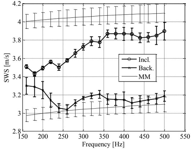
Fig. 4. SWS estimation (m/s) of a heterogeneous phantom of 10% and 8% for inclusion and background region with their respective mechanical measurements.
