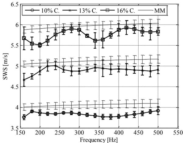
Fig. 3. SWS estimation obtained from WAVE method in homogenous phantom of 10%, 13%, and 16% gelatin concentration with their respective mechanical measurements.
