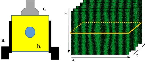
Fig. 1. Left side: Conventional crawling wave setup. (a) Vibration source, (b) examined tissue, (c) probe. Right: sonoelasticity video showing the interference pattern produced by the vibration sources. WAVE is computed over each depth slice across the lateral and temporal dimension to generate an SWS image.
