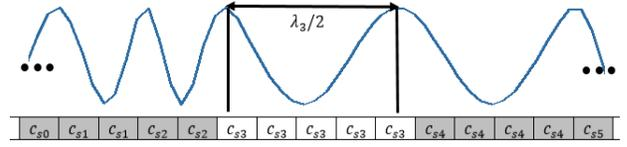
Fig. 2. Interference pattern along the lateral dimension at a selected depth and frame, and its estimated partial SWS vector. The distance between peaks represent half the wavelength of the average SWS.
