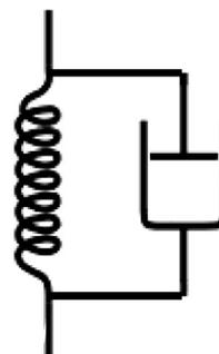
Fig. 8. The Kelvin-Voigt parallel spring-dashpot model in mechanics has some of the properties of the coincident stiffness and viscosity assigned to the elements of an idealized viscoelastic medium. A parallel mass is implied.
