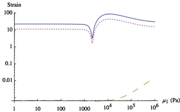
Fig. 6. Normalized, absolute value of the strains on the axis of a translationally oscillating sphere: radial longitudinal strain,  $S_{rr}$  (solid); transverse strain,  $S_{\theta\theta}$ ,  $S_{\phi\phi}$  (dotted); dilatational strain,  $S_{rr} + 2S_{\theta\theta} = \Delta V/V$  (dashed line). All parameters are as used in Fig. 1 except  $\theta = 0$ .
