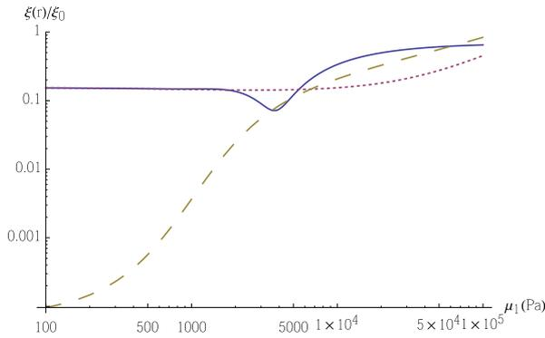
Fig. 2. Absolute value of the radial component of the displacement. All parameters are the same as in Figure 1, except  $\theta = 0$ .
