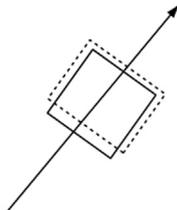
Fig. 5. Shear strain resulting from a radially oscillating bubble. The amplitude,  $A$ , is a strong function of the distance from the bubble. The shape of a cubical element morphs to that of a rectangular cuboid. When the radial component of the element contracts, the polar and azimuthal components expand, keeping the volume of the element approximately constant.
