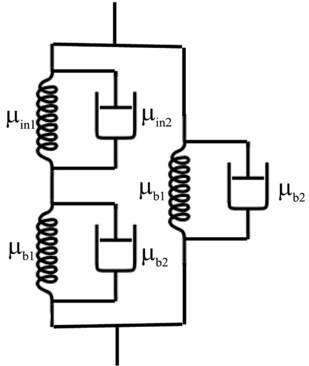
Fig. 12. Relaxation model. Stress is transferred through a portion of the bulk medium to an internal system.
