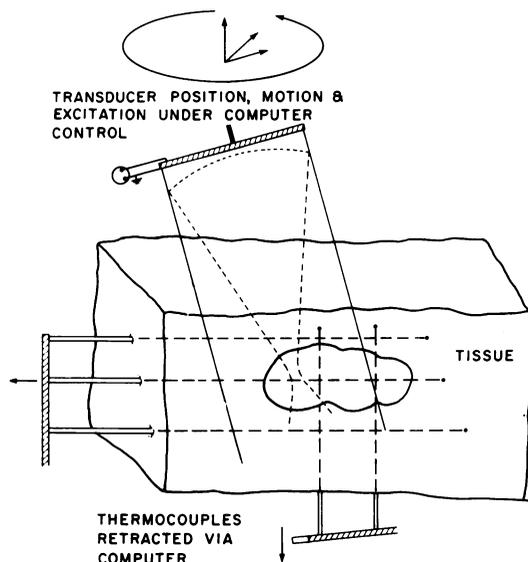
FIG. 2.—Insonation head positioning and thermocouple "stepping" system.
