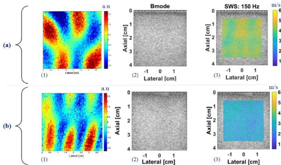
**Figure 3:** RSW experimental results on phantom with: (a) 7% gelatin and 12% castor oil, (b) 5% gelatin and 12% castor oil. (1) shows the RSW field generated within the phantom at the frequency of 150Hz, (2) is the B-scan, (3) demonstrates the SWS map obtained from the AC estimator at 150Hz overlaid on the B-scan.
