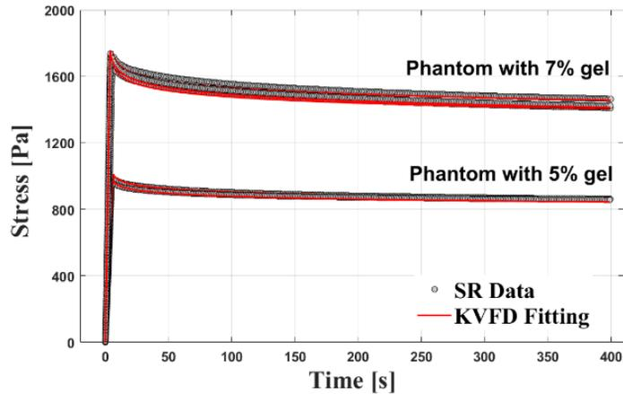
**Figure 4:** SR results on different samples from the two phantoms fitted to the KVFD model.
