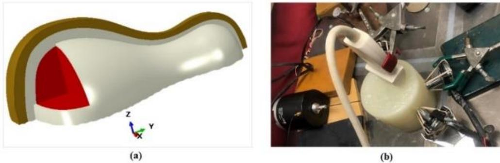
**Figure 1:** (a) 3D model of liver (red color) surrounded by a layer of fat (cream color) and muscle (brown color) for FE simulations. (b) Experimental set-up for RSW experiment on a phantom with 7% gelatin and 12% castor oil.
