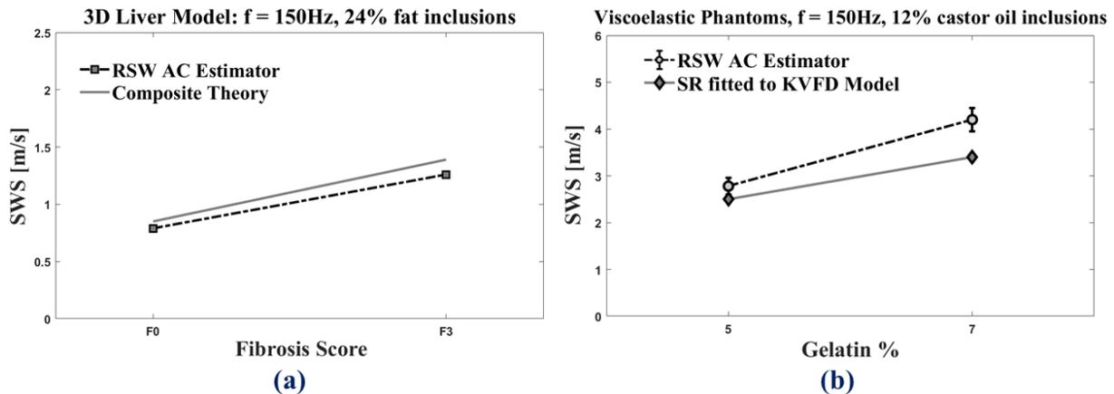
**Figure 5:** (a) Comparison of SWS from RSW simulations with the theory of composite theory. (b) Comparison of SWS from RSW experiments on phantoms with the SWS from SR tests on phantoms as an independent test.
