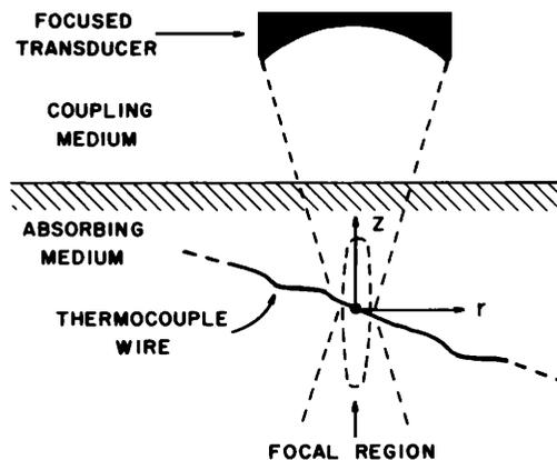
FIG. 2. The positioning of a focused beam over an embedded thermojunction for absorption measurements.
