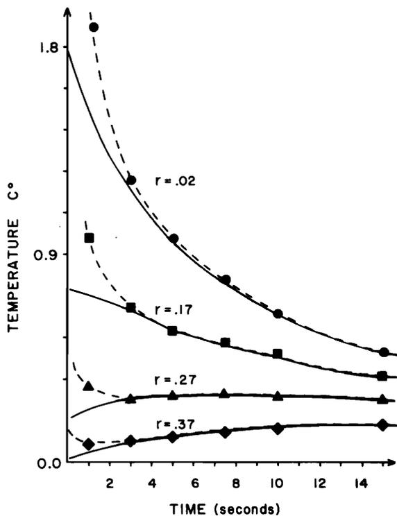
FIG. 6. Temperature histories in an absorbing medium, following a 0.06-s pulse of ultrasound, using the off-axis pulse-decay method. Dotted lines—experimental results. Solid lines—theory, neglecting the viscous heating component.  $r$  = the lateral displacement of the focal region relative to the thermojunction, in cm.
