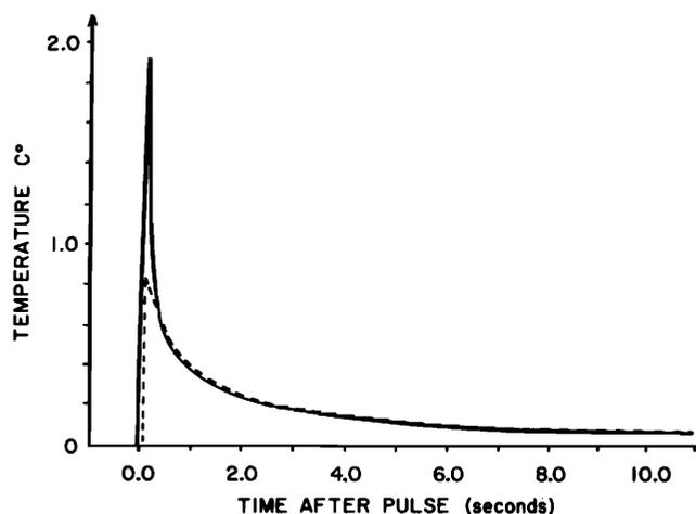
FIG. 3. The temperature history following a 0.08-s ultrasonic pulse. Solid line—measured temperature. Dotted line—curve fit of theory (neglecting viscous heating component) to data in the interval of 2 to 10 s. By the extrapolation back to time  $t = 0$ , the heating caused by absorption alone is determined.
