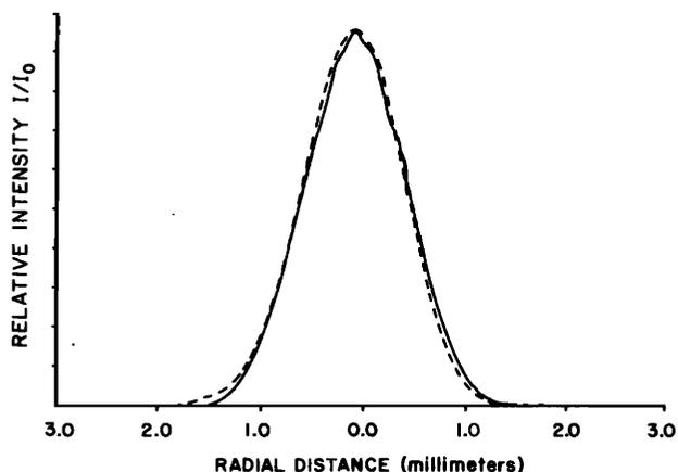
FIG. 1. Intensity of a 2.7-MHz focused beam. Solid line—measured at 0.1-mm increments. Dotted line—least squares error Gaussian curve fit.
