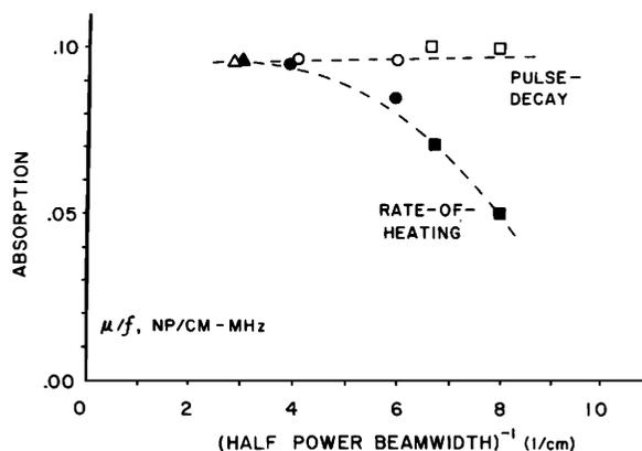
FIG. 4. The absorption coefficient of beef liver samples as a function of beamwidth using the pulse-decay and rate-of-heating methods. The rate-of-heating method does not account for heat loss by conduction and produces low estimates of absorption when small beamwidths are used. Triangles—0.9 MHz. Circles—1.8 MHz. Squares—2.7 MHz.
