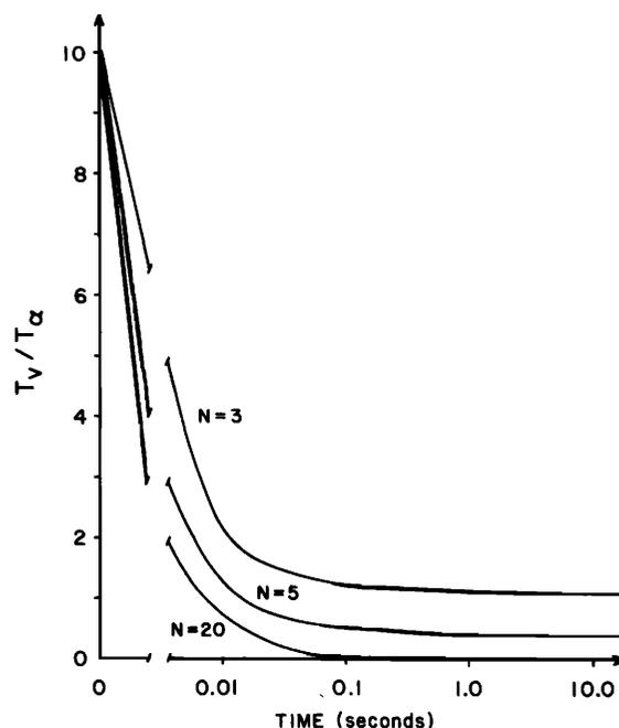
FIG. 5. The ratio of elevated temperatures caused by viscous heating effects, to heating from absorption, using typical parameters.  $N$  is the ratio of beam width to thermocouple diameter.
