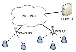
Figure 1. A traditional mobile computing topology. Users are connected to a remote cloud server through a 3G/4G Base Station (BS) or a WiFi Access Point (AP).
