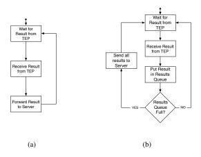
Figure 4. Result collection flowcharts for the TDP operating according to the *Proxy* (a) and *Batch* (b) methods.
