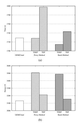
Figure 5. Time (a) and energy consumption (b) for computing 50 tasks, for a systems where only 1 node is allowed to execute the tasks. "TEP" refers to the the performance of a TEP that receives the tasks from a local TDP.
