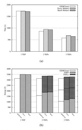
Figure 6. Time (a) and energy consumption (b) for computing 50 tasks, when 1, 2 and 3 nodes are allowed to execute the tasks. For the proxy and batch methods, the case "1 TEP" refers to a system with one TDEP. For multiple TEPs, the contributions of the different devices is also presented.
