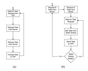
Figure 3. Task distribution flowcharts for the TDP operating according to the *Proxy* (a) and *Batch* (b) methods.
