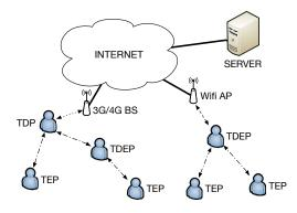
Figure 2. Example of ad hoc mobile computing topology with corresponding functional role assigned to each of the clients. Task distribution point (TDP), task execution point (TEP), and task distribution and execution point (TDEP).
