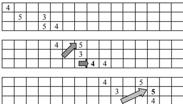
Figure 3: Traffic Behaviors of highway traffic model. Integers represent the velocities of the vehicles.
