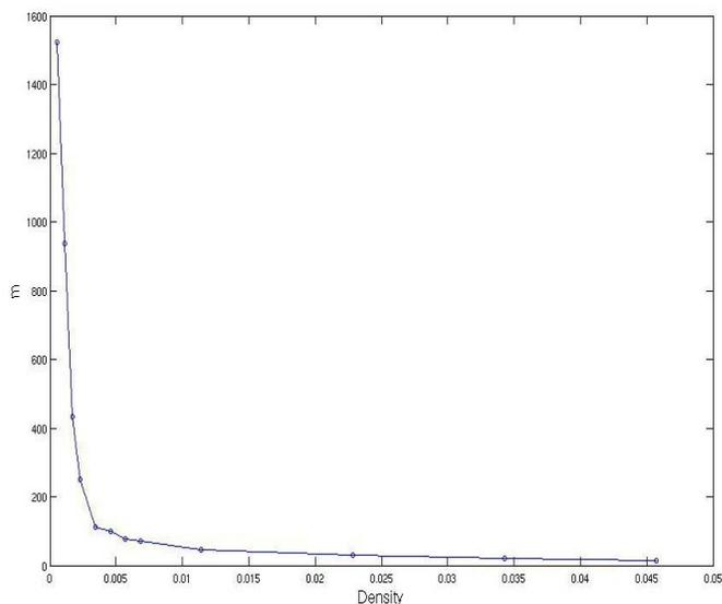
Figure 10: Distance to closest moving car vs. per lane density on a 3-lane highway.
