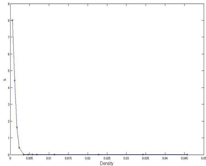
Figure 8: Minimum delay from accident vs. per lane density for a 3-lane highway.
