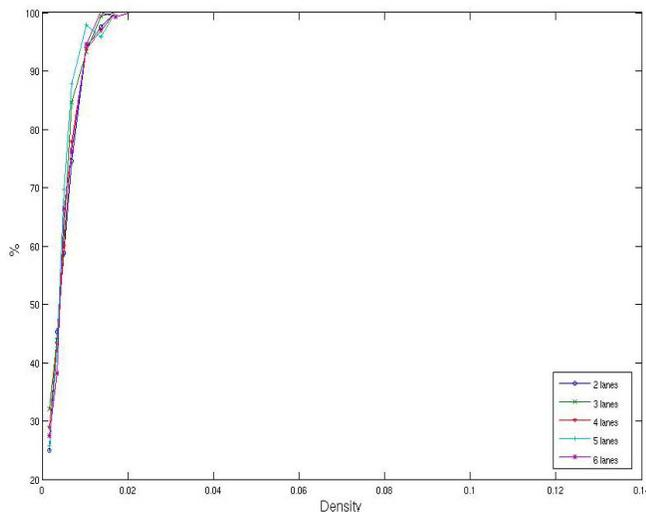
Figure 5: Max PDR vs. Density for 2-to-6 lane bidirectional highways. All nodes receive at least one notification packet for a density of at least 0.017.
