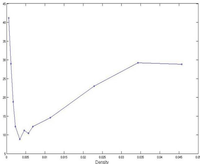
Figure 7: Average Number of Dropped Packets vs. per lane density on a 3-lane highway
