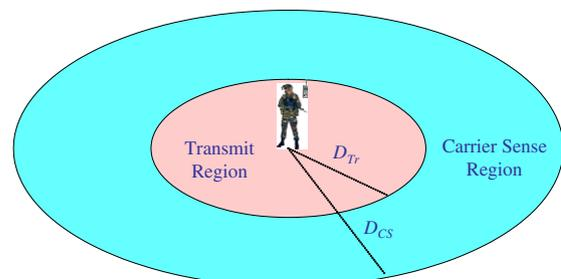
Fig. 2. Illustration of transmit and carrier sense regions.
