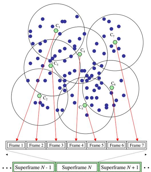
Fig. 6. A snapshot of MH-TRACE clustering and medium access for a portion of an actual distribution of mobile nodes. Nodes C1–C7 are clusterhead nodes.
