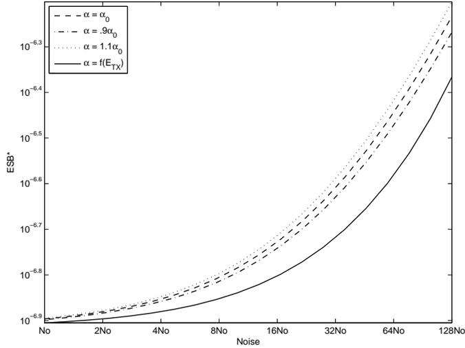
Figure 4.8:  $ESB$  as a function of amplifier efficiency
