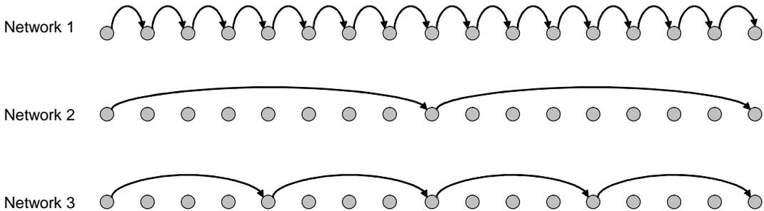
Figure 1.1: Three examples of a linear wireless network. Network 1 has a short hop distance, Network 2 has a long hop distance, and Network 3 has the optimal hop distance.
