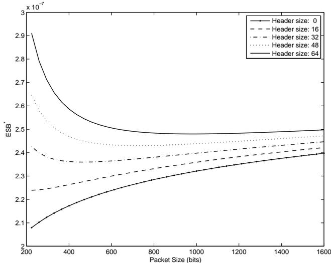
Figure 4.7: Effect of packet size on the  $ESB$
