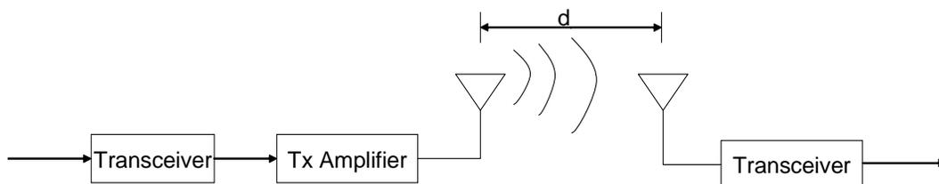
Figure 3.1: Wireless channel system model.
