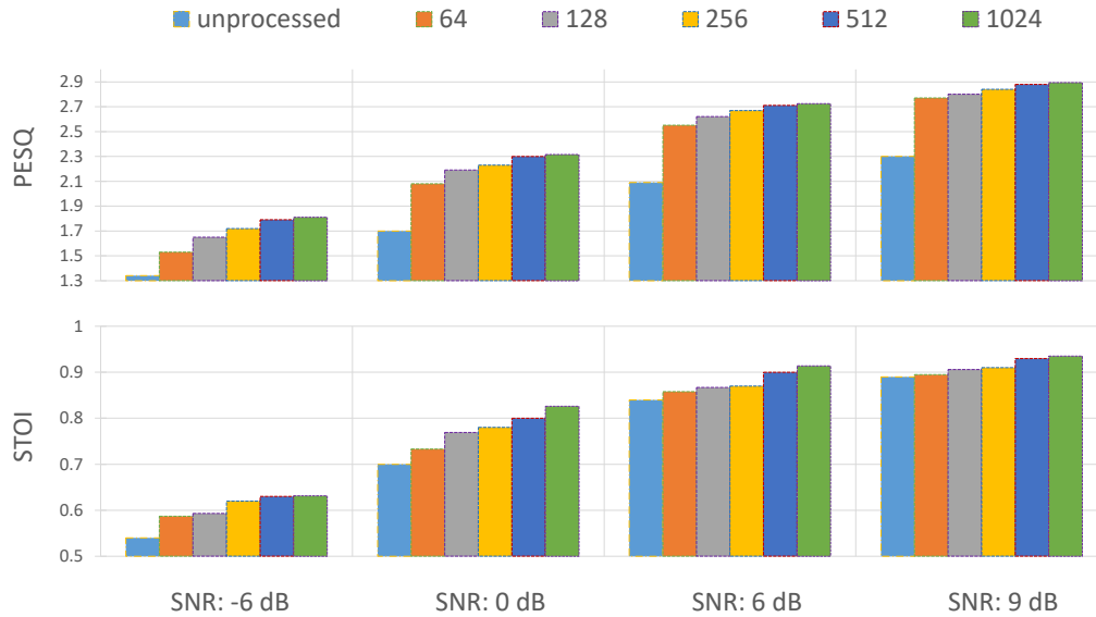
Figure 2.7: PESQ and STOI comparisons averaged over all noise types for different numbers of hidden units (64, 128, 256, 512 and 1024) per layer in the BLSTM network.
