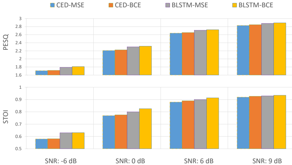
Figure 2.11: PESQ and STOI comparisons averaged over all noise types for mean-squared error (MSE) and binary cross-entropy (BCE) loss functions in BLSTM and CED networks.
