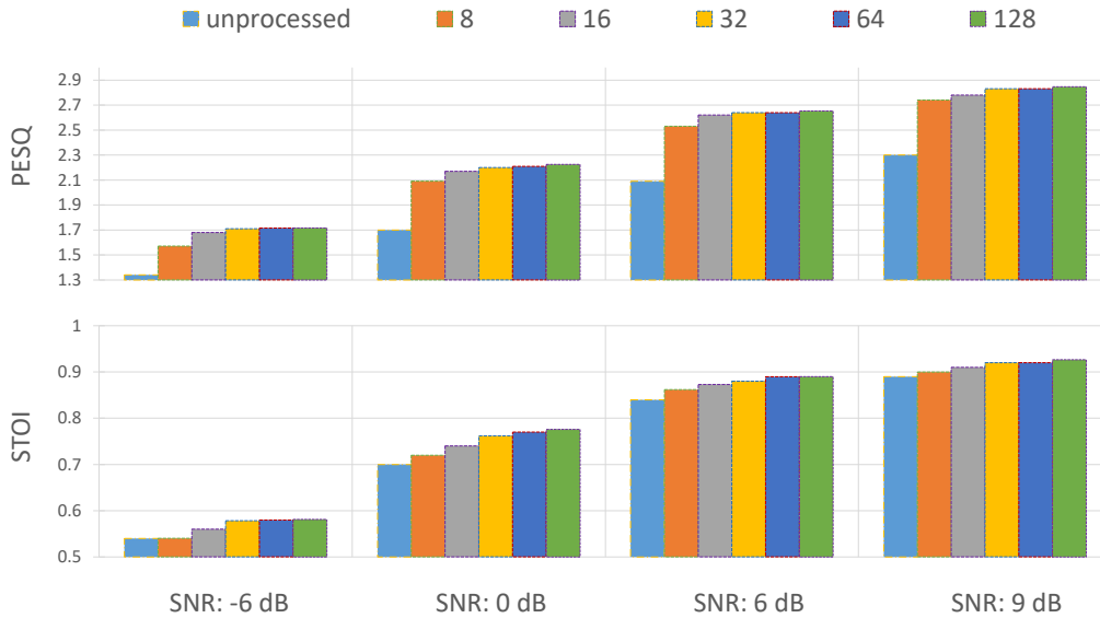
Figure 2.8: PESQ and STOI comparisons averaged over all noise types for different numbers of filters ( M = 8, 16, 32, 64 and 128 ) in the first convolutional layer in the CED network. The numbers of filters in the other convolutional and deconvolutional layers are powers-of-two times of M , following the same symmetric pattern shown in Fig. 2.2.
