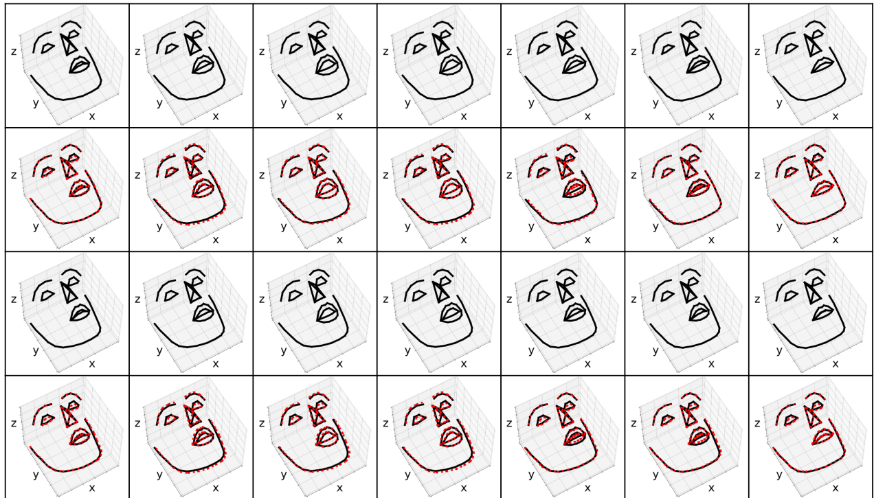
Figure 3.11: The example output showing the pronunciation of the word “ash”. The speech sample was taken from STEVI corpus. The first row shows the result generated by ID_CNN . The second row shows the comparison of the result generated by ID_CNN and the ground-truth (dotted red line). The third and fourth rows show the result generated by ID_CNN_TC and comparison with the ground-truth (dotted red line). Columns show every three frames.
