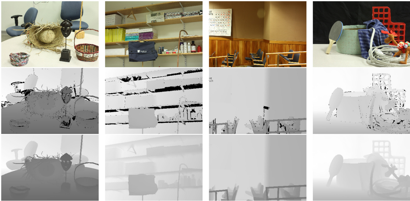
Fig. 3 Visual results demonstrating the hole-filling ability of the proposed algorithm on a subset of images from the Middlebury stereo dataset 2014. 30 The first row shows the input high-resolution color images and the second row shows the corresponding depth maps. The results are shown in the last row. The illustration in this figure has used input images with approximately 60 to 80 k pixels.
