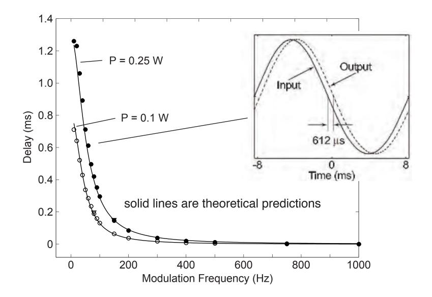
For 1.2 ms delay, v = 60 m/s and  $n_g = 5 \times 10^6$
