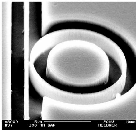
Figure 5. Example of a ring resonator fabricated in GaAs.
