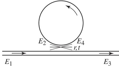
Figure 1. Optical disc resonator coupled to an optical waveguide.
