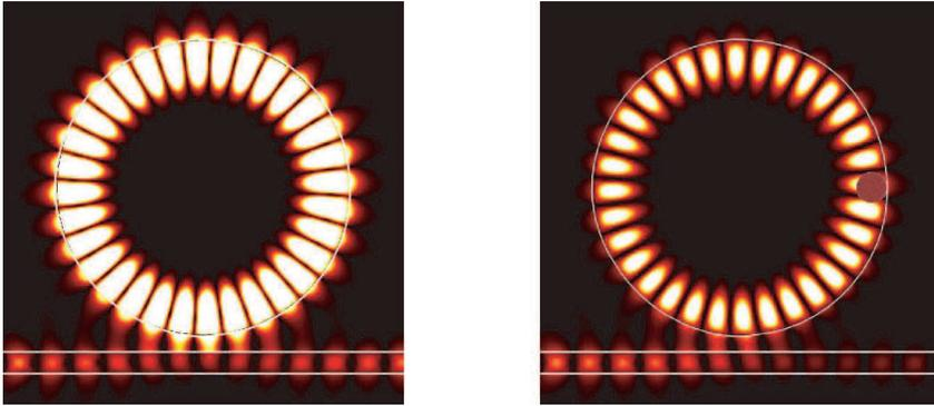
Figure 6. Conceptual design of a disc resonator photonic biosensor. The upper surface of the disc resonator is coated with a layer of binding material. When a pathogen falls onto this surface it is selectively bound to it, producing to an increased loss mechanism that leads to decreased transmission.
