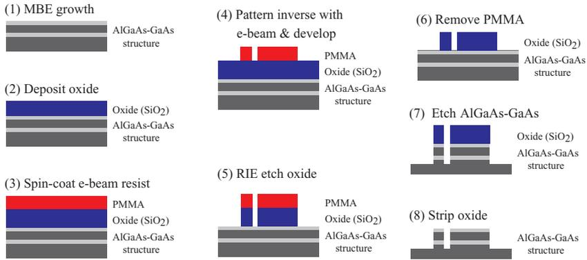
Figure 4. Fabrication procedure used in the manufacture of the photonic devices. MBE = molecular beam epitaxy, CAIBE = chemically assisted ion beam etch, PMMA = poly methyl methacrylate.
