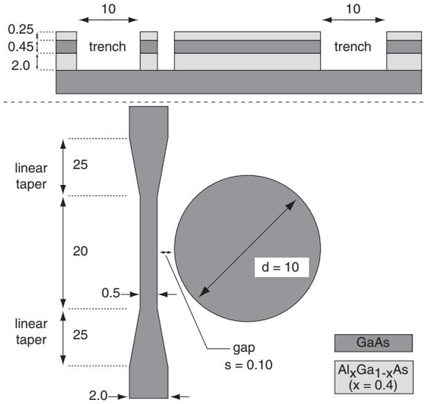
Figure 3. Design of the basic disc resonator structure.
