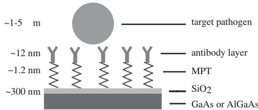
Figure 7. Laboratory procedure for selective binding of biological materials onto a GaAs or AlGaAs substrate.
