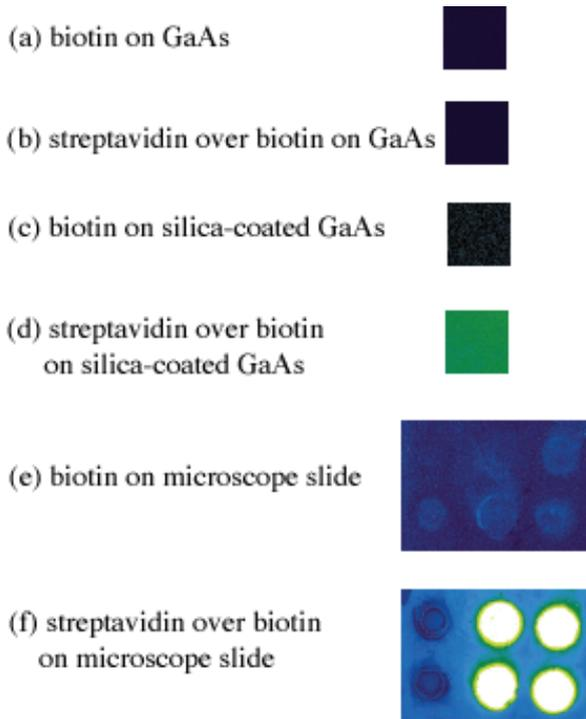
Figure 8. Laboratory demonstration showing selective binding of a biological material onto a GaAs substrate.
