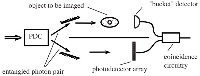
Figure 1. A typical ghost imaging setup.
