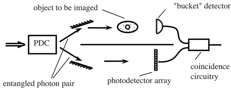
Figure 1. A typical ghost imaging setup.
