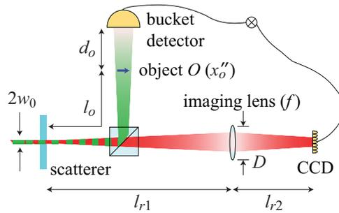
Figure 3. Geometry of two-color ghost imaging.
