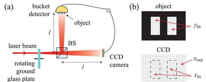
Fig. 1. (Color online) (a) Schematic representation of lensless thermal ghost imaging. (b) Simplified object model for analysis. The object plane (upper) and the reference detector plane (lower) are discretized by pixels of finite sizes. The light falling on a pixel is assumed to be statistically independent of that on other pixels.
