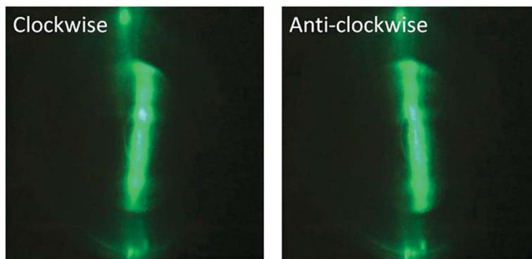
**Fig. 1.** An intense line of laser light is focused through a 100-mm-long ruby rod. The images show the transmitted intensity as recorded on a screen positioned  $\sim 500$  mm behind the rod spinning at  $\pm 30$  Hz. The difference in line orientation between the two directions is  $\sim 10^\circ$ . The fixed light at the top and bottom of the images is transmitted around the sides of the ruby and hence not subject to any rotation.
