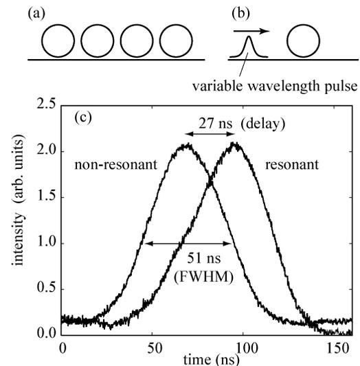
Fig. 6. (a) A ring-resonator optical delay line. (b) One element of the delay line. (c) Demonstration of controllable optical time delay in the setup of (b). A 51-ns pulse is delayed by 27 ns.
