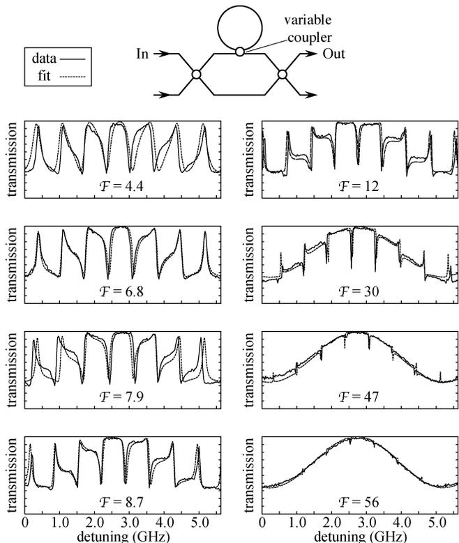
Fig. 4. Measured transmission spectra of a nearly balanced Mach-Zehnder interferometer with the 31-cm fiber ring resonator inserted into one arm. The setup is shown at the top. Data were taken near  $1.55 \mu\text{m}$  for the same coupler settings as in Fig. 3. The dotted lines are a theoretical fit to the data.
