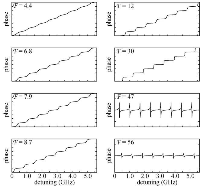
Fig. 5. Spectral dependence of the phase shift acquired by a light wave in interacting with the fiber ring resonator as determined from the fits to the data shown in Fig. 4. For better visibility, the vertical gradations are in units of  $2\pi$  for the first six overcoupled resonator plots and units of  $\pi/6$  for the remaining two plots.
