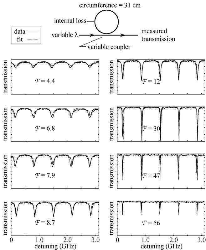
Fig. 3. Measured transmission spectra near  $1.55 \mu\text{m}$  for a fiber ring resonator 31 cm in circumference with nonnegligible loss for a variety of coupler settings. The setup used to perform the measurement is shown at the top. The dotted lines are a theoretical fits to the data. The resonator is overcoupled, critically coupled, and undercoupled for  $\mathcal{F}$  less than, equal to, and greater than 30, respectively.
