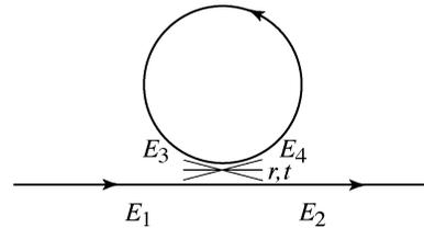
Fig. 1. Geometry of a fiber ring resonator.
