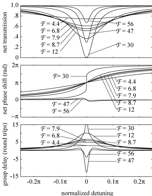
Fig. 2. Theoretically predicted net transmission, phase shift, and group delay for an ideal ring resonator with single-pass transmissivity  $\tau = 0.95$  and varying values of the finesse. The normalized detuning is the angular frequency difference between the light field and the nearest cavity resonance multiplied by the ring circulation time.
