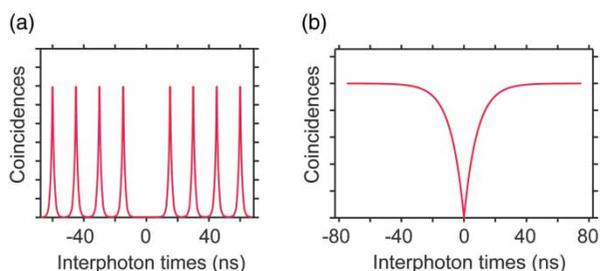
Figure 11. Photon antibunching histograms with dips at zero times for pulsed laser excitation (a) and for cw laser excitation (b). These histograms show how many second photons in consecutive photons pairs appear after first photons at definite time intervals (coincidences). The second-order correlation function  $g^{(2)}(t)$  is proportional to coincidence count.
