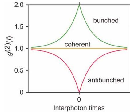
Figure 3. Dependence of a second-order coherence function  $g^{(2)}(t)$  on an interphoton time  $t$  for light sources with different photon statistics.
