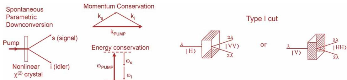
Figure 8. Spontaneous parametric down conversion: Left – schematics and conservation of energy and momentum. Right – type I interaction (signal and idler photons have the same linear polarizations).
