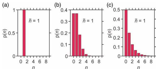
Figure 2. Photon number ( $n$ ) probability distribution [ $P(n)$ ] for photon sources with different statistics, but with the same mean photon number  $\bar{n} = 1$ . (a) Single (antibunched) photon source (Fock state); (b) laser (coherent) light; and (c) thermal source.
