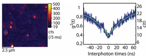
Figure 15. Left: Confocal fluorescence microscopy image of single CdSeTe NQDs in a glassy CLC photonic bandgap microcavity. Right: Raw coincidence counts  $c(t)$  (right-hand scale) and  $g^{(2)}(t)$  (left-hand scale), showing antibunching (dip at  $t = 0$ ). (Reproduced with permission [29]).
