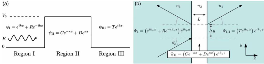
Figure 9. (a) Tunneling in quantum mechanics: a particle of energy  $E$  encounters a potential barrier of height  $V_0$ . (b) An optical analog to (a): a photon undergoes FTIR.
