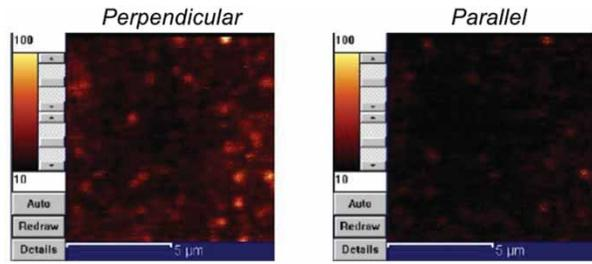
Figure 21. Confocal fluorescence microscopy images of DiI dye single-molecule fluorescence in a planar-aligned, glassy, nematic LC host ( $10 \times 10 \mu\text{m}$  raster scan). Left: Polarization perpendicular to the alignment direction; right: parallel polarization. Scale shows counts/pixel.
