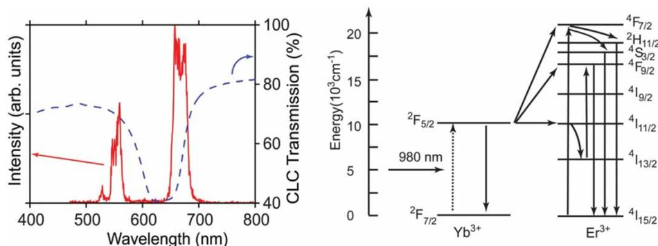
Figure 24. Left: Red solid lines: Fluorescence spectrum of  $\text{Er}^{3+}$  ions doped in  $\text{NaYF}_4$  nanocrystals dispersed in a chiral CLC microcavity (E7 and CB15). The blue dashed curve shows the spectral transmission of CLC microcavity measured with unpolarized light. Right: Energy levels of  $\text{Er}^{3+}$  and  $\text{Yb}^{3+}$  and upconversion excitation scheme under 980 nm excitation.
