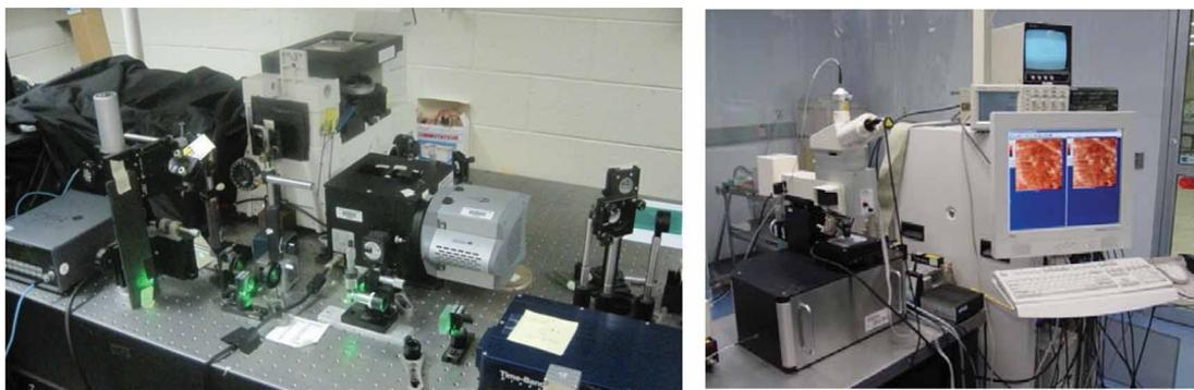
Figure 12. Two single-photon generation, detection, and characterization units used in experiments: Left – a home-made confocal fluorescence microscope with different diagnostics; Right – an alpha-SNOM WITec microscope comprising confocal, near-field, and an atomic force microscope with a Hanbury Brown and Twiss set up for antibunching measurements.
