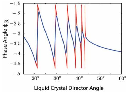
Figure 28. The predicted phase of the reflection coefficient based on the  $4 \times 4$  matrix method described in the text for 727-nm light incident on an 8- $\mu\text{m}$  LC cell. The parameters used are  $\theta = 63.5^\circ$ ,  $n_{\text{glass}} = 1.77$ ,  $n_e = 1.63$ , and  $n_o = 1.54$ . The resulting phase is then convolved with a Gaussian function to account for a spread of input  $k$ -vectors (blue solid line).
