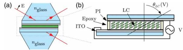
Figure 27. Diagram of the double-prism structure. In (a) a LC cell is sandwiched between two equilateral glass prisms. An exploded diagram of the LC cell is shown in (b). The substrates are coated with transparent ITO electrodes to facilitate electronic control of the LC molecular director rotation angle  $\theta_{LC}$ , and thin PI to aid the alignment of the LC layer. (Reproduced with permission [41]).
