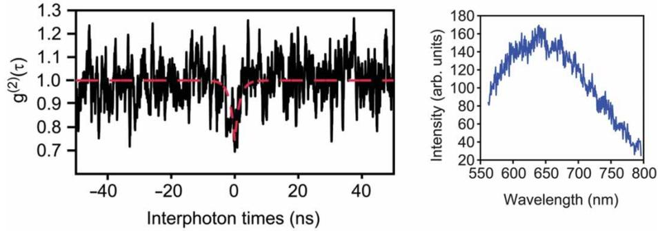
Figure 25. Left: Photon antibunching from NV center nanodiamond in a monomeric CLC host. Black curve shows the raw data. Red dashed curve shows the fit. Right: Fluorescence spectrum of NV centers in nanodiamonds in a monomeric CLC host (cw, 514-nm laser excitation).
