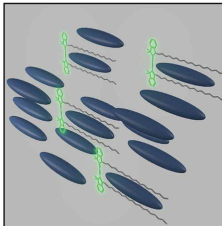
Figure 20. Schematic view of DiI dye molecules in a nematic LC host. The long axis (alkyl chains) of the DiI molecules tend to orient themselves along the rod-like nematic molecules, while the dipole, which is parallel to the bridge between the alkyl chains, orients perpendicular to the direction of LC alignment.
