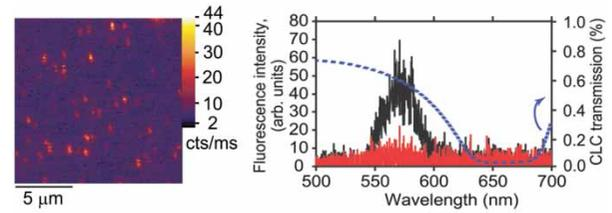
Figure 16. Left: Confocal fluorescence microscopy image of single CdSe NQDs in a monomeric CLC photonic bandgap microcavity. Right: Fluorescence spectrum of CdSe NQDs in the monomeric planar-aligned CLC host for two different circular polarizations of single photons (Black curve of high intensity – right handed – and red curve – left handed). CLC selective transmission curve is shown by a dashed blue line.
