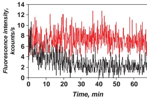
Figure 6. Fluorescence bleaching behavior of an assembly of terrylene dye molecules as a function of time for oxygen-depleted LC (red curve) and for LC without special oxygen depletion (black curve).
