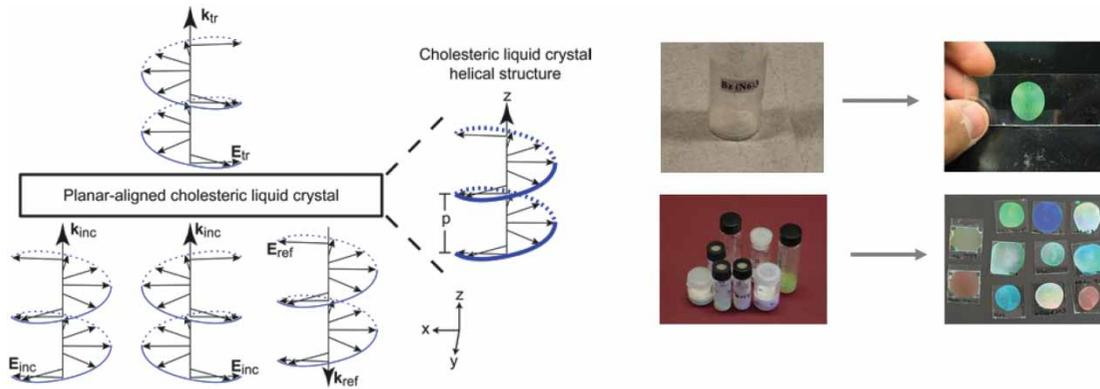
Figure 13. Left: Circular polarized light propagation in a 1-D photonic bandgap CLC structure. Right: Preparation of photonic bandgap CLC structures from a powder oligomer (top) and monomeric LCs (bottom).
