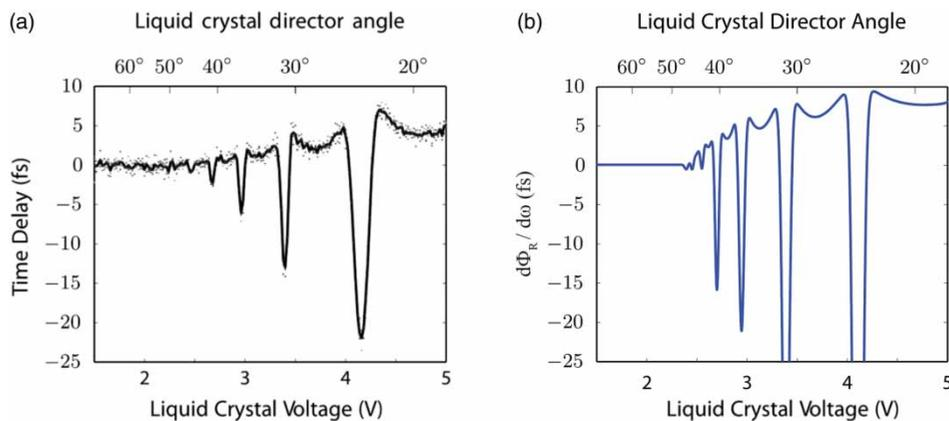
Figure 31. (a) Reflection delay in FTIR from the double-prism structure. The black line is the arithmetic mean of four individual data-sets. Each data point represents an individual Hong–Ou–Mandel trace with 102 seconds of integration time. (b) Predicted  $d\phi_R/d\omega$  for 727-nm light propagating through an 8- $\mu\text{m}$  LC cell. (Reproduced with permission [41]).
