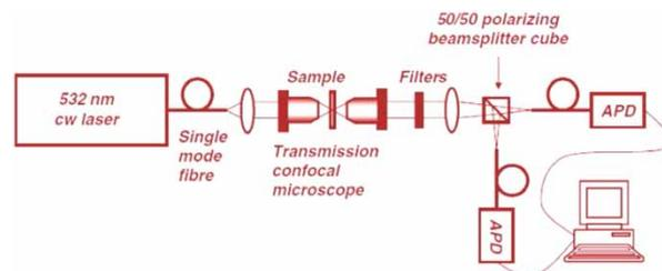
Figure 19. Experimental set up for polarization measurements using a modified WITec microscope (Figure 12, right).
