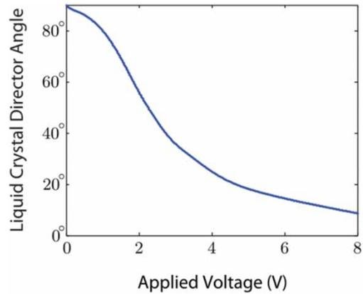
Figure 29. Dependence of the LC molecular director angle on applied voltage obtained from transmission measurements. We did not measure a pretilt angle, so  $90^\circ$  in the plot is an approximate value.
