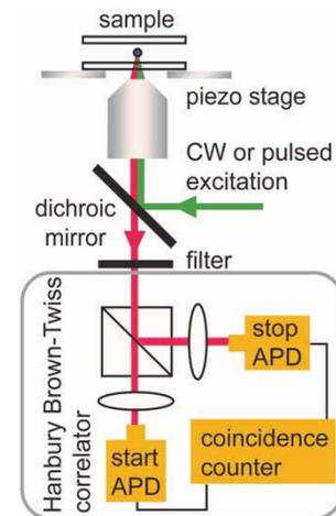
Figure 10. Schematic of a single-photon generation, detection, and characterization unit (APD – single-photon counting avalanche photodiode module). A Hanbury Brown and Twiss correlator is used for photon antibunching measurements.
