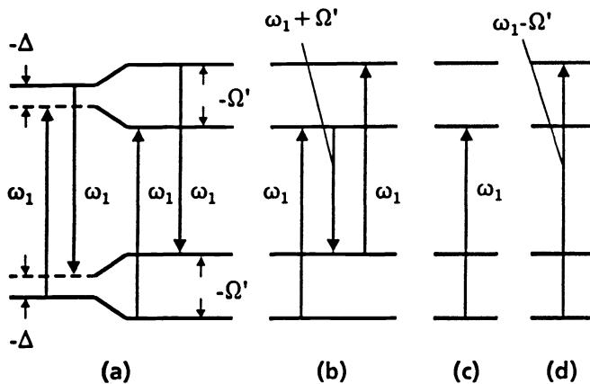
Figure 10. (a) In the presence of a strong, nearly resonant optical field, the ground and excited states of an atom are split into doublets separated by the generalized Rabi frequency  $\Omega'$ . The transitions (b-d) between the modified levels correspond to the resonances in the absorption spectrum shown in Fig. 11.
