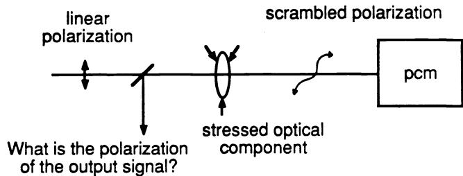
Figure 1. Diagram showing schematic experimental setup to study the polarization characteristics of phase conjugation.
