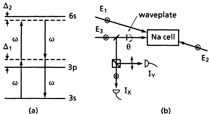
Figure 7. (a) Energy-level diagram showing the two-photon resonantly enhanced DFWM process. (b) Experimental setup used to study VPC by two-photon-resonant DFWM.
