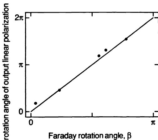
Figure 5. Rotation angle of the polarization vector of linearly polarized radiation after reflection from a vector phase conjugate mirror and retraversal through a Faraday rotator plotted as a function of the rotation angle  $\beta$  of the Faraday rotator.
