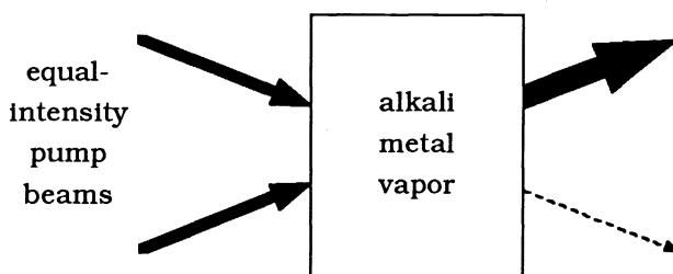
Figure 9. Nonlinear interactions can be utilized to coherently combine two input beams into a single output beam which contains nearly all of the incident power.
