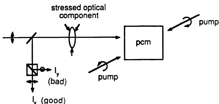
Figure 2. Experimental setup used to demonstrate polarization aberration correction by four-wave mixing using circularly polarized, counter-rotating pump beams.
