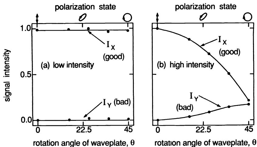
Figure 8. Intensity of each polarization component plotted as a function of the degree of polarization distortion introduced into the probe wave. (a) For low pump intensities the effects of the polarization distortion are removed essentially completely. (b) For high pump intensities, severe degradation of the VPC process is observed.
