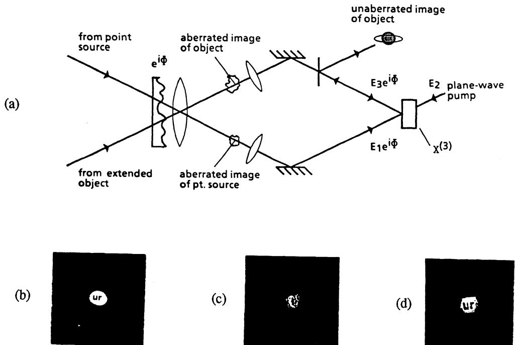
Figure 6. (a) Schematic experimental arrangement for passive, one-way phase-aberration correction using four-wave mixing. (b)-(c) Photographs demonstrating aberration correction using four-wave mixing. The input image (b) is severely aberrated (c) by a phase distorter. The restored image (d) is recovered on the other side of the aberrator from the original object.
