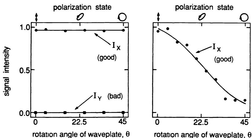
Figure 4. Intensities of each polarization component plotted as a function of the degree of polarization distortion introduced into the probe wave. (a) For circularly polarized, counter-rotating pump beams, the effects of the polarization distortion are removed essentially completely ( $I_x \gg I_y$  and  $I_x$  is independent of  $\theta$ ) (b) For circularly polarized, corotating pump beams, the quality of VPC is severely degraded ( $I_x$  and  $I_y$  are comparable and depend on  $\theta$ ).
