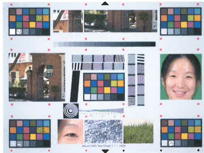
Fig. 2(a) The reference image simulated with an ideal lens. The lens has no aberrations; Strehl ratio of 1. The sensor has 3 million pixels, size 1.75\mu\text{m} .
