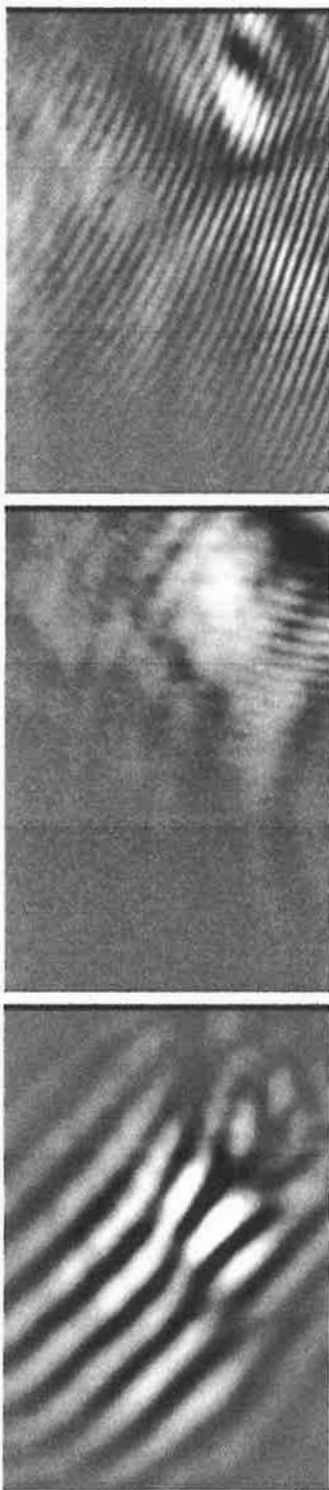
Fig. 2. Coarse-frequency fringes for two beam holographic system at 10.6 \mu m, shown in Fig. 1.
