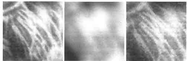
Figure 10. Expanded view of whiskers: left, logarithmic asphere at 950 mm; right, logarithmic asphere at 700 mm; centre, Nikon at 700 mm.
