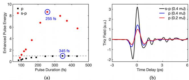
**FIG. 4.** (a) The dependence of the THz pulse energy on the pulse duration. The black squares represent the single-pump excitation case. The red dot shows the result of double pump excitation. The time delay between two pumps is 6.8 ps. With the same total laser pulse energy, the THz energy is enhanced by 8.6 times. (b) The corresponding THz waveforms when the time delay is 255 fs.
