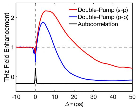
**FIG. 3.** The dependence of the THz field peak field on  $\Delta\tau$  (red and blue lines). The black line is the result of the autocorrelation measurement, which is employed to determine the 0 time.  $\Delta\tau > 0$  means that the prepump ionizes liquid water first.
