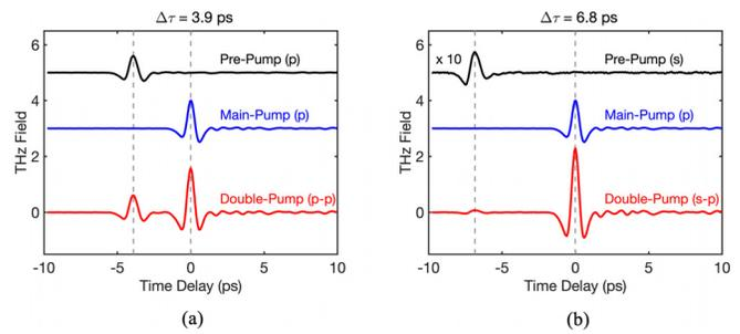
**FIG. 2.** THz wave generation enhanced by a preformed plasma. (a) THz signals individually generated by the p-polarized prepump and main-pump are plotted as the top and middle lines. The bottom line shows the THz signal generated by two beams with a certain time delay  $\Delta\tau$ . (b) Similar results are plotted when the prepump is s-polarized. The enhancement is greater than (a), where the prepump is p-polarized. All the signals are normalized by the signal from the p-polarized main-pump.
