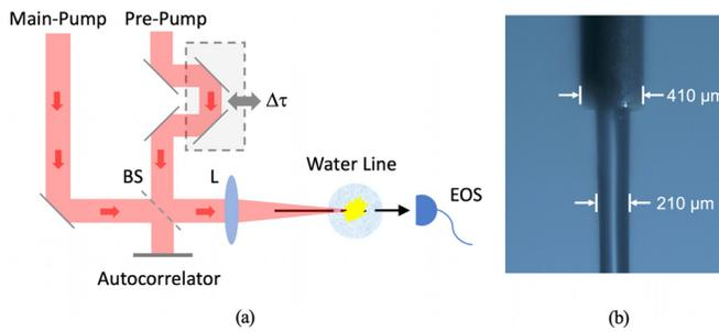
**FIG. 1.** Experimental setup. (a) Two collinearly propagating main- and prepump beams are focused by a lens to ionize a water line (top view). The time delay ( $\Delta\tau$ ) between two optical pumps is controlled by a translation stage. The THz signal is detected through electro-optical sampling (EOS) in the forward direction. Additionally, the pulse duration is monitored by an optical autocorrelator. (b) A photo of a 210  $\mu\text{m}$  water line (side view).
