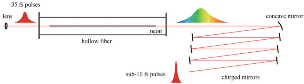
**Fig. 24** Schematics of hollow fiber pulse compressor used in our experiment. 35 fs second laser pulses was input into a hollow core fiber placed in a neon-filled chamber. The self-phase modulation of intense laser pulses provides a sufficient bandwidth. Output pulses are compressed down to sub-10 fs by three pairs of chirped mirrors
