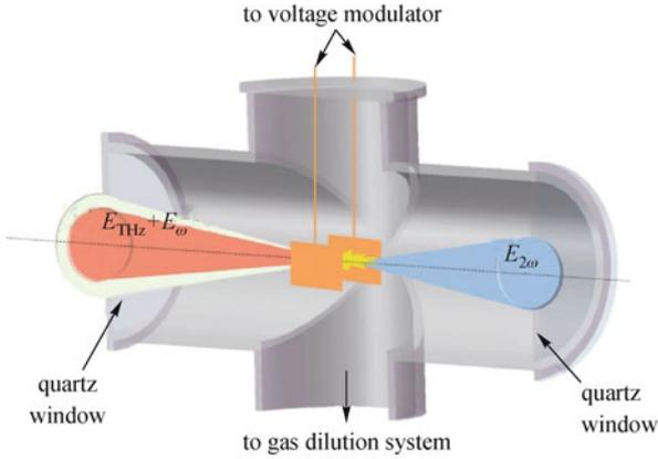
**Fig. 2** Schematic illustration of gas cell. Both the entrance and exit windows were made of quartz, which is relatively transparent to both fundamental and second harmonic beams. The quartz material has low absorption at the frequency below 5 THz. The electrical field was connected through an electrical feed-through at the top of gas cell and the gases were introduced through the bottom of the cell
