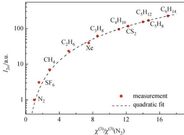
**Fig. 6** Detected second harmonic intensity ( $I_{2\omega}$ ) versus third order nonlinear susceptibility ( $\chi^{(3)}$ ) of gases. Red dots are experimental data and black dashed line is the quadratic fit. Y-axis is normalized with the reference signal taken with 100 torr nitrogen gas at the same experimental condition. Also, all the  $\chi^{(3)}$  are normalized with that of nitrogen
