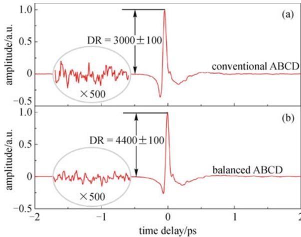
**Fig. 22** Comparison of measured dynamic ranges (DRs) between (a) conventional ABCD and (b) balanced ABCD. Background fluctuations with a 500 times magnification are shown in gray circles. Waveforms are normalized with peak values. Waveforms are obtained with a lock-in time constant of 100 ms and a total of 9 scans
