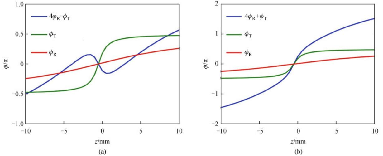
**Fig. 11** Calculated Gouy phase shift corresponding to (a)  $\omega + \omega - \Omega$  and (b)  $\omega + \omega + \Omega$  process during ABCD.  $z$  is the longitudinal position along beams' propagation direction. Zero position is the focus position. Rayleigh ranges of terahertz beam and optical probe beam are 0.8 and 4.8 mm, respectively. Green, red and blue curves represent the phase change of terahertz waves, optical beams and phase difference between the two, respectively
