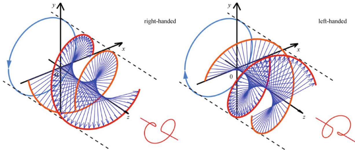
**Fig. 30** Illustration of double helix electrical field applied on plasma region. Laser pulses are focused to ionize air where a pair of double helix electrodes was positioned. The trajectory of electrons follows the direction of external electrical field, resulting in an elliptically polarized terahertz wave in far field. The laboratory coordinate and definition of handedness are shown in the figure
