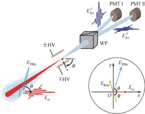
**Fig. 19** Schematic of balanced ABCD for terahertz waves. WP: Wollaston prism. PMT: photomultiplier tube. The polarization of each beam and the experimental coordinate are shown inside the gray circle
