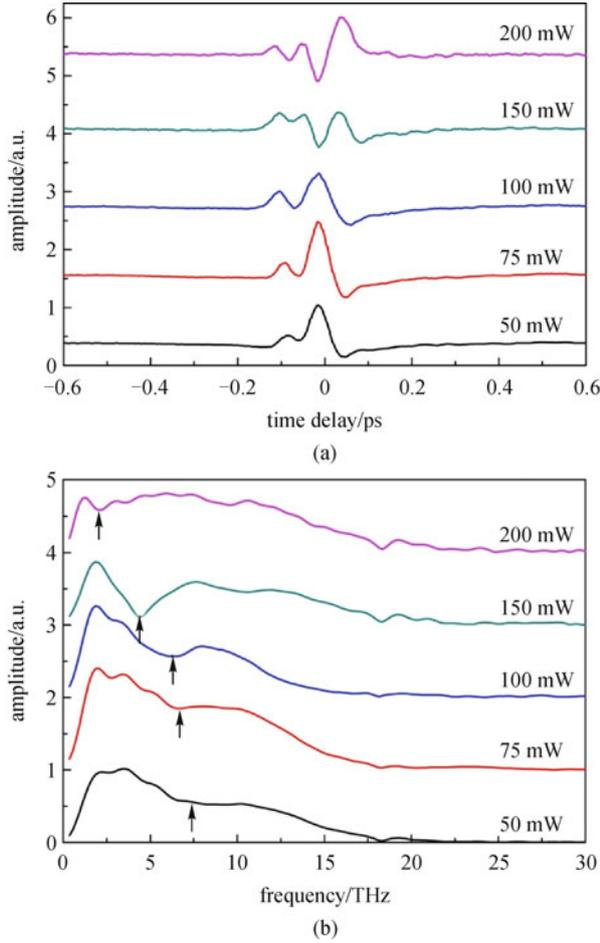
**Fig. 4** Terahertz (a) waveforms and (b) spectra obtained with different probe pulse energy. Electrodes were placed around the center of plasma. Black arrows are the guides for the absorption frequency, which shows a red shift while increasing the probe pulse energy
