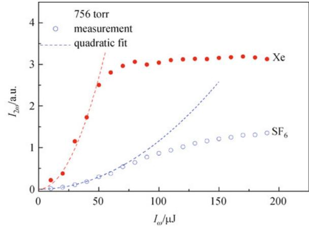
**Fig. 3** Measured second harmonic intensity ( $I_{2\omega}$ ) versus the probe pulse energy ( $I_{\omega}$ ) at a bias field of 7.5 kV/cm, and gas pressure of 756 torr with Xe and SF<sub>6</sub> gases. Dots are from measurements and dashed lines are quadratic fits. The deviation of the probe energy dependence above 50  $\mu$ J for Xe and 70  $\mu$ J for SF<sub>6</sub> are consistent with the onset of intensity clamping due to plasma formation
