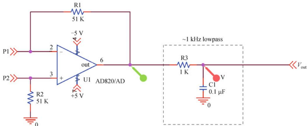
**Fig. 20** A circuit diagram of current subtractor. Current outputs from two PMTs (P1 and P2) are sent through an analogy device AD 820, which can provide a output proportional to the subtraction between P1 and P2 (Courtesy Dr. Brian Schulkin)
