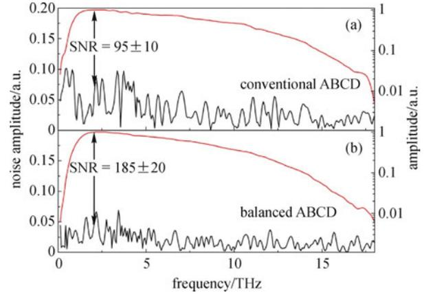
**Fig. 23** Comparison of measured signal-to-noise ratio (SNR) between (a) conventional ABCD and (b) balanced ABCD. Terahertz spectra and noise floors are shown in red and black lines, respectively. Signals were obtained with a lock-in time constant of 100 ms and a total of 9 scans
