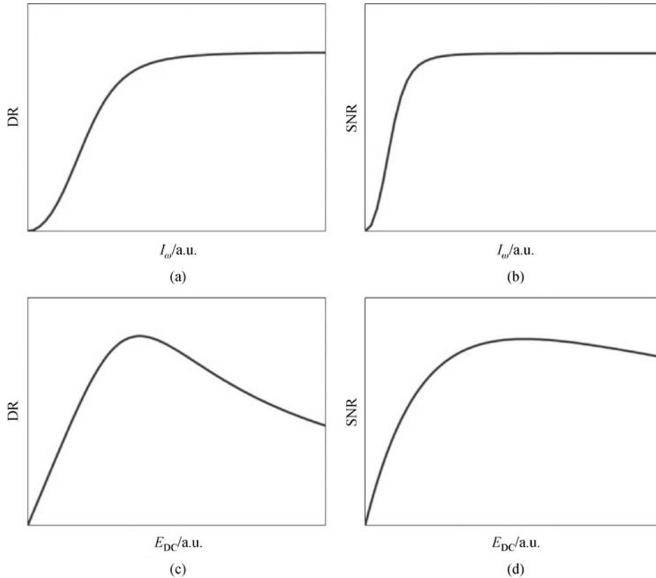
**Fig. 15** Calculated trend of (a) and (c) dynamic range (DR); (b) and (d) signal-to-noise ratio (SNR) with respect to (a) and (b) probe pulse energy ( $I_\omega$ ); (c) and (d) DC field strength ( $E_{DC}$ ) in ABCD system
