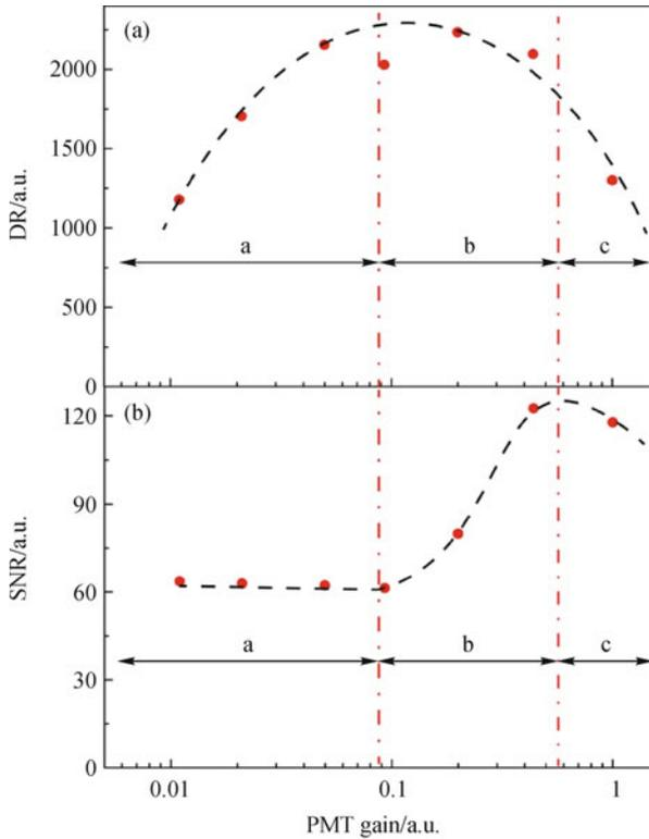
**Fig. 17** Comparison of (a) dynamic range (DR) and (b) signal-to-noise ratio (SNR) with respect to the gain of PMT. Red dots are measured experimental data and dashed black curves are the guide for the eye
