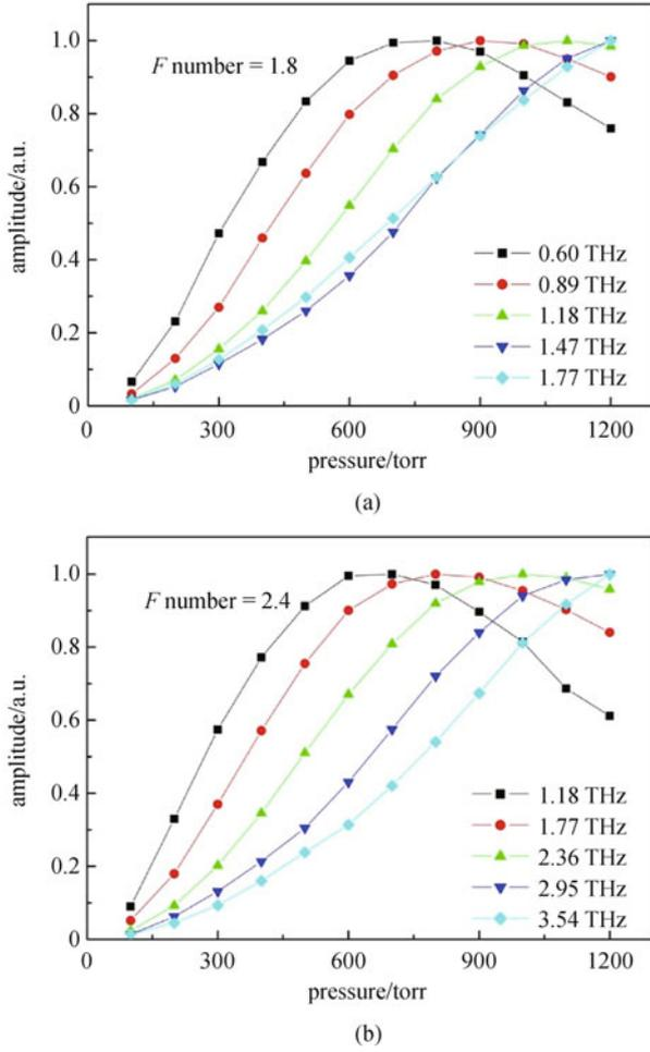
**Fig. 9** Pressure dependence of various frequency components with Xe sensor at (a)  $F$  number = 1.8 and (b)  $F$  number = 2.4. The probe beam power is 20 mW and bias field strength is about 8 kV/cm. Data were normalized with peak value for clarity
