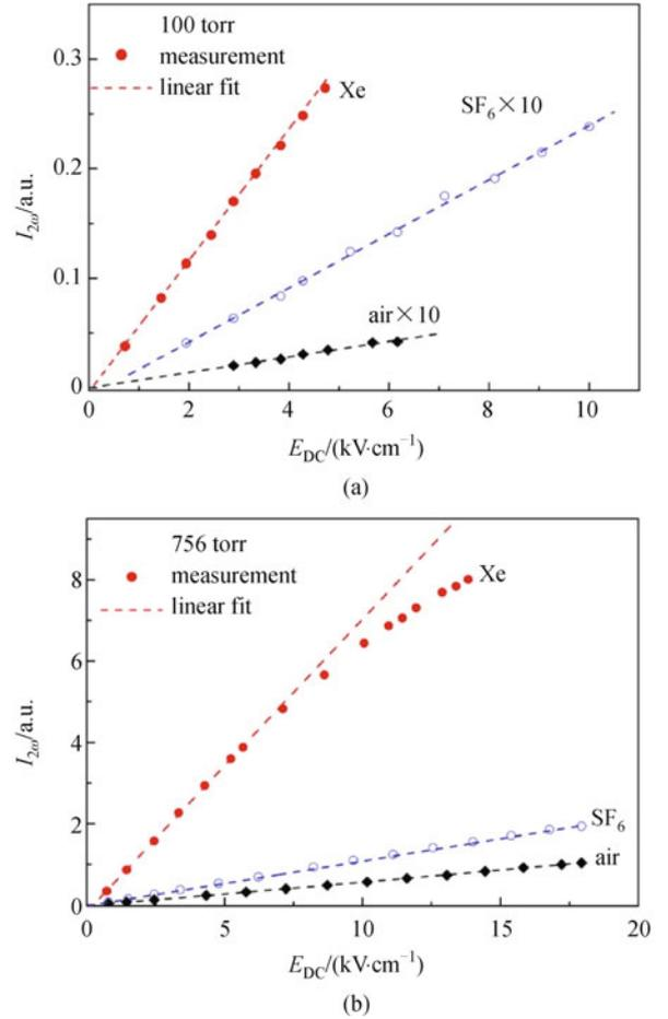
**Fig. 5** Measured second harmonic intensity ( $I_{2\omega}$ ) versus DC bias field ( $E_{DC}$ ) at gas pressure of (a) 100 torr and (b) 756 torr, with a probe pulse energy of  $50 \mu J$ . Dots are from measurements and dashed lines are linear fits
