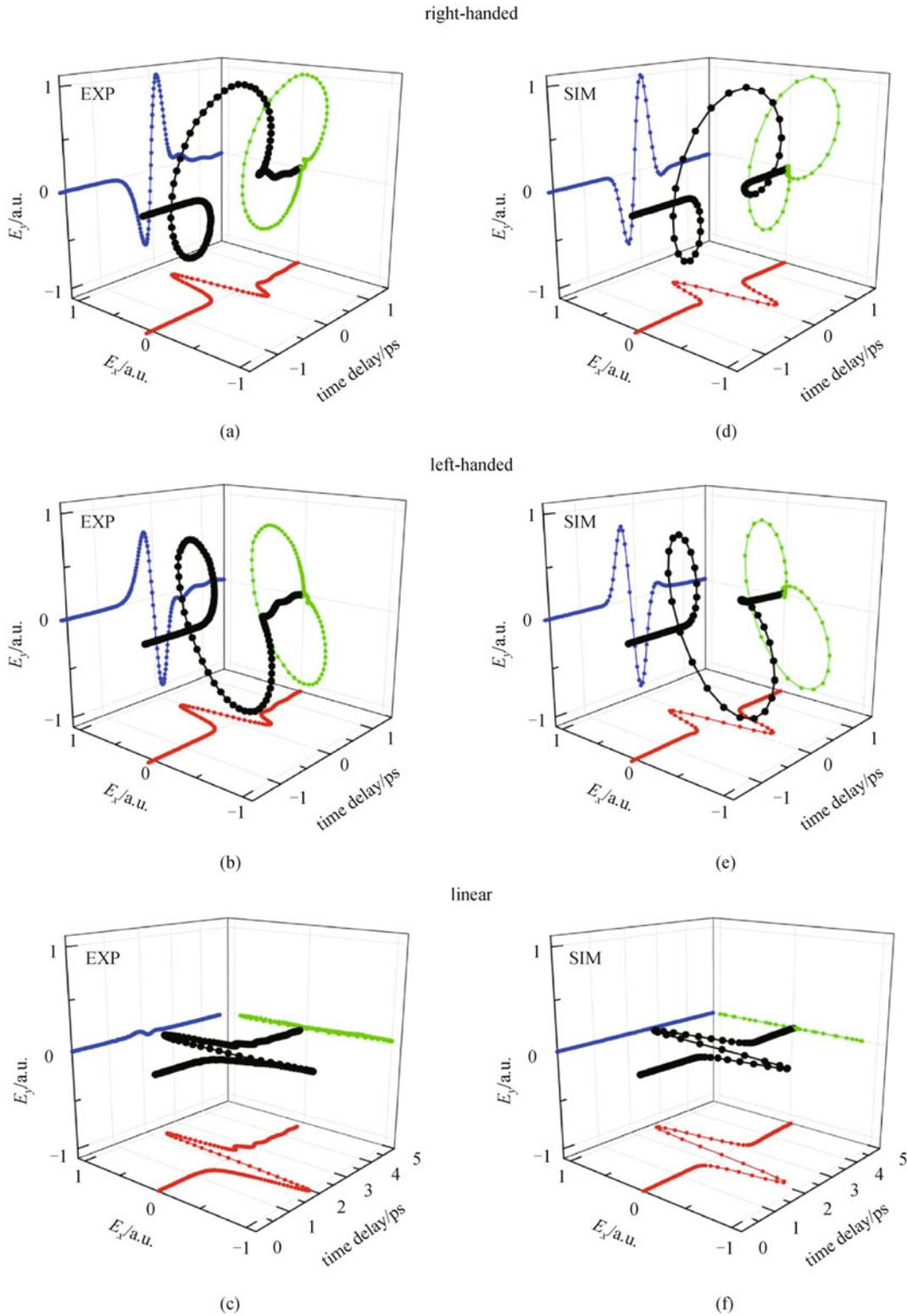
**Fig. 31** Temporal evolution of electrical field vector of (a) right-handed and (b) left-handed elliptically polarized and (c) linear polarized terahertz pulses. Simulated temporal evolution of electrical field vector of (d) right-handed and (e) left-handed elliptically polarized and (f) linear polarized terahertz pulses. EXP: experimental results. SIM: simulation results
