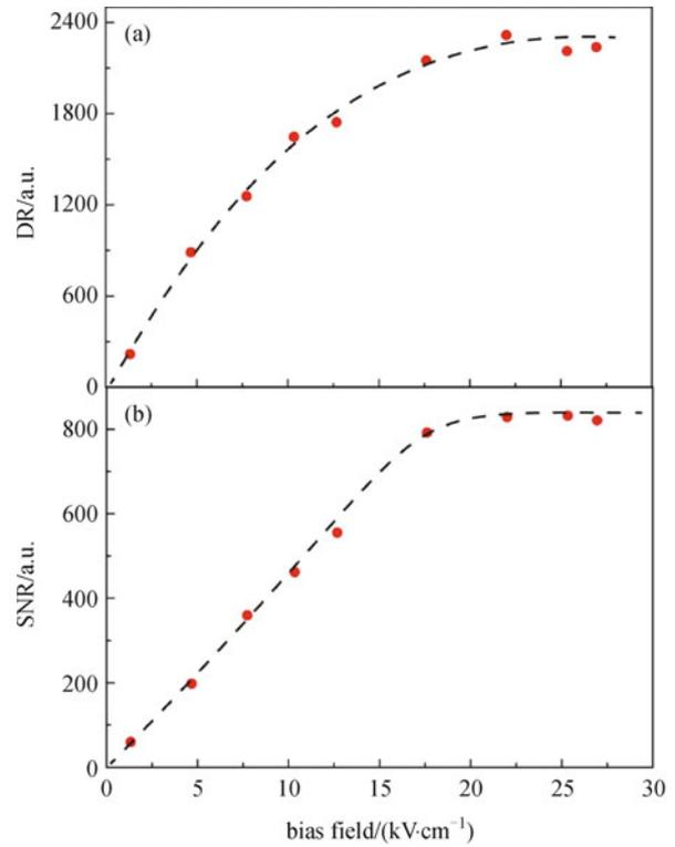
**Fig. 18** Comparison of (a) dynamic range (DR) and (b) signal-to-noise ratio (SNR) with respect to bias field strength. Blacked dashed lines are the guides for the eyes
