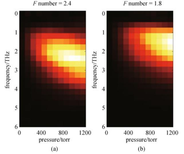
**Fig. 8** 2D plot of detected terahertz spectra with Xe versus pressure at different terahertz focus condition. The terahertz Rayleigh lengths without and with iris were estimated to be 0.8 and 1.5 mm, respectively. The different phase match of each frequency component results in a spectral shift toward high frequency. (a)  $F$  number = 2.4; (b)  $F$  number = 1.8
