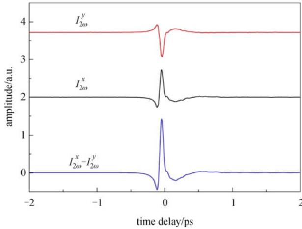
**Fig. 21** Each component measured in balanced ABCD. Waveforms are offset vertically for clarity
