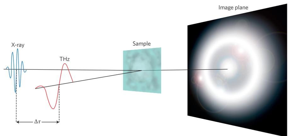
**Figure 1** | Conceptual illustration of a pump-probe experiment employing a THz pump and an X-ray probe for time-resolved nanoscale imaging. The idea is to use the THz pulse as a pump to modify the atomic structure of a target and then capture an image of the atomic structure by X-ray scattering.  $\Delta\tau$  is the timing between the X-ray pulse and the THz pulse.
