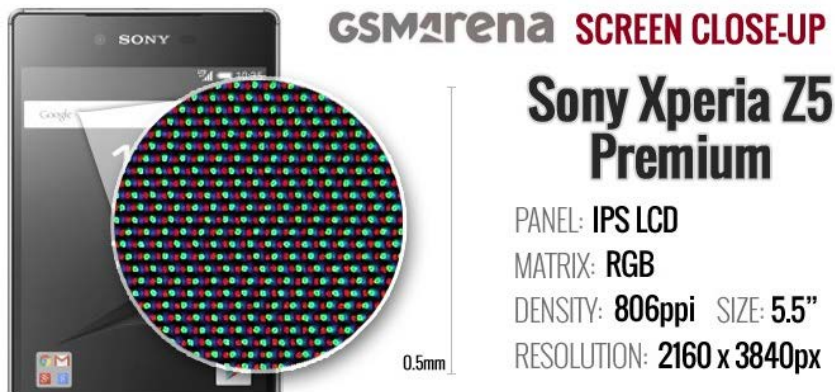
Figure 3. Pixel arrangement of Xperia Z5 Screen. This layout is not an accurate representation of the RGB pixel distribution.
