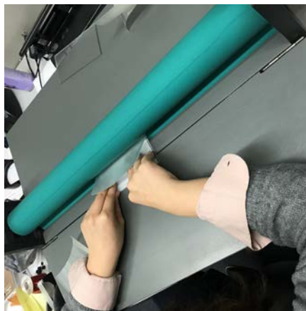
Figure 10. Adhering a lenslet array to an acrylic board using a roller.
