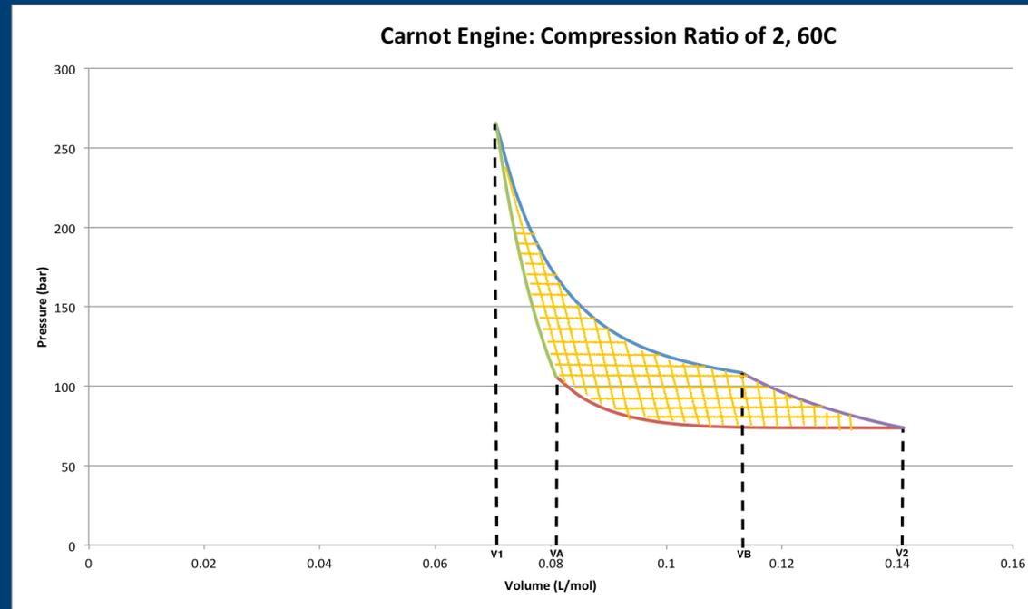
Figure 2: Carnot Cycle on P-V Plot
