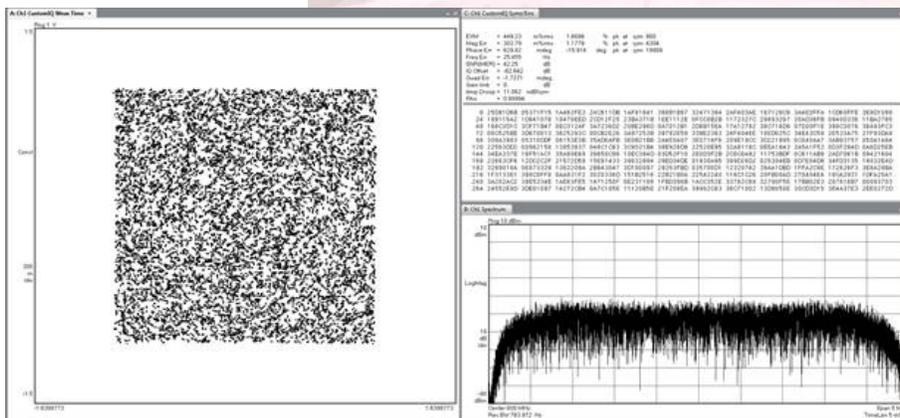
Figure 1. Demodulation of a 16384-QAM with 0.45% EVM with 400mW average power – measurement performed using a signal using a Keysight MXA model N9020A
