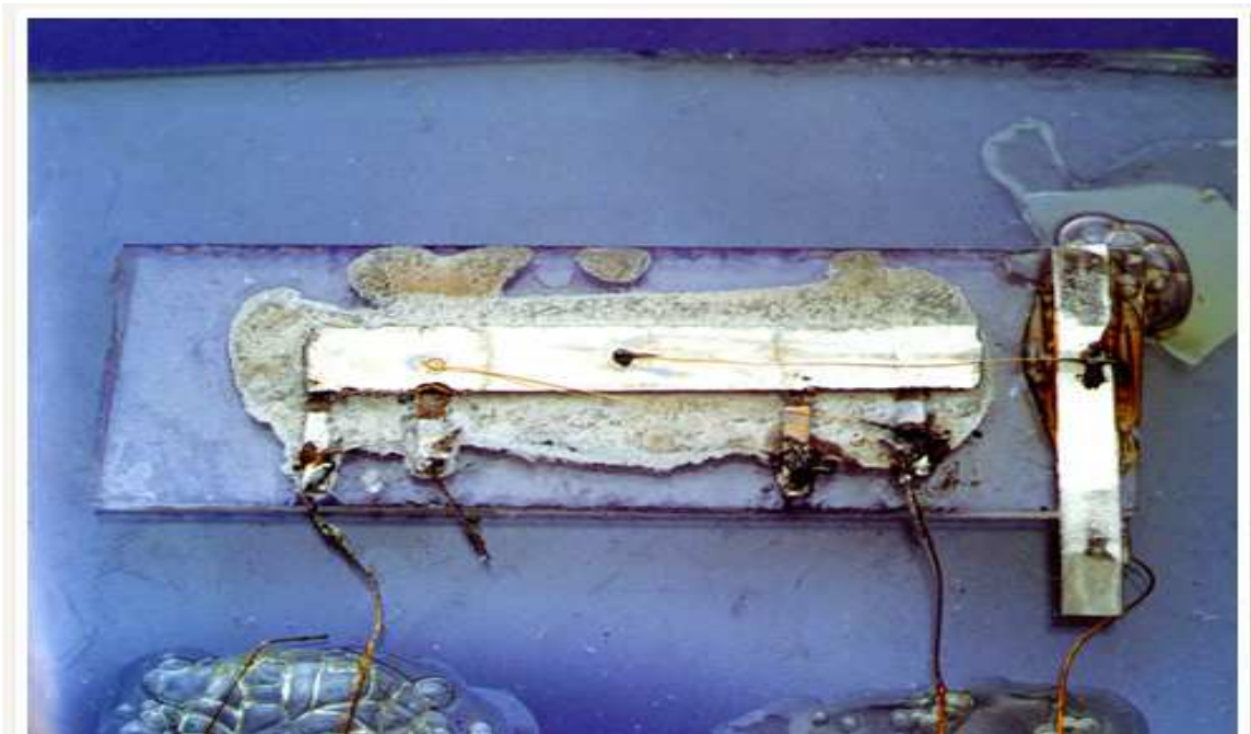
Figure 1.2: The first integrated circuit developed by Jack Kilby at Texas Instruments in 1958 [3].
