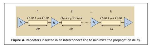
Including resistance in the interconnect model dramatically changed the design and analysis of integrated circuits. With a short circuit or a capacitive interconnect model, the interconnect could be treated as a single node.
