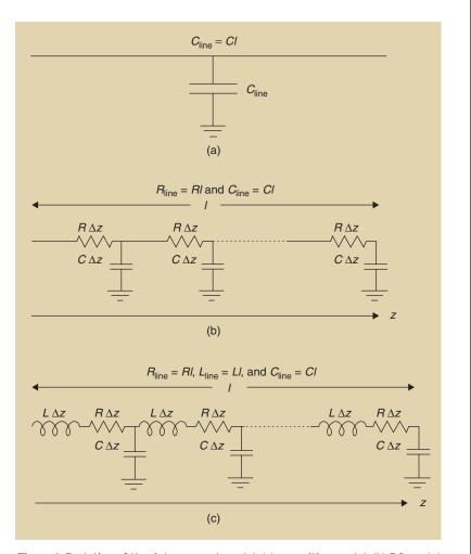
**Figure 1.** Evolution of the interconnect model: (a) capacitive model; (b) RC model; (c) RLC model.
