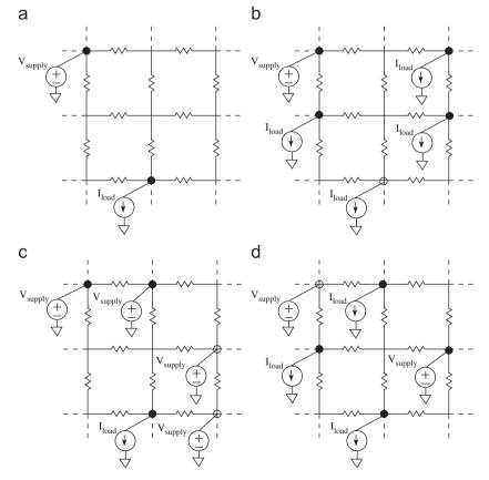
Fig. 2. Simplified power grid models with (a) one voltage source and one current load, (b) one voltage source and multiple current loads, (c) multiple voltage sources and one current load, and (d) multiple voltage sources and multiple current loads.
