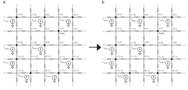
Fig. 9. Power distribution grid model (a) multiple power supplies and current loads are connected to several nodes and (b) all but one of the voltage sources are replaced with an equivalent current source.
