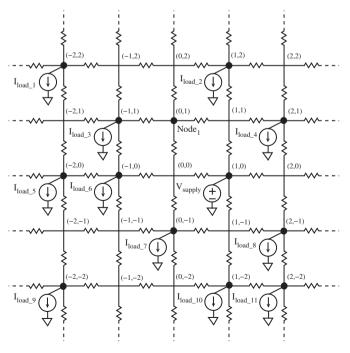
**Fig. 5.** Model of power distribution grid when one power supply is connected to node (1,0) and multiple current loads model the load circuits connected at various nodes within the power distribution grid.
