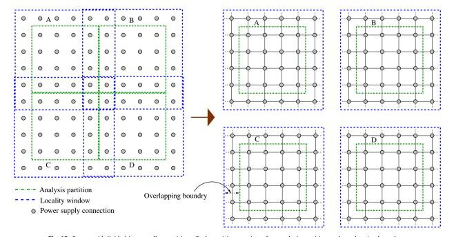
Fig. 15. Power grid divided into smaller partitions. Each partition consists of an analysis partition and overlapping boundary.
