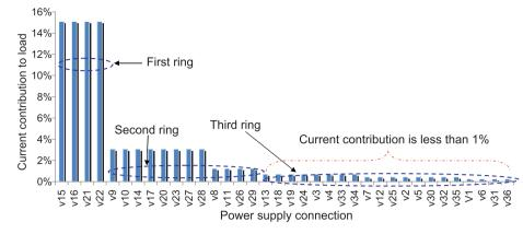
**Fig. 12.** Percent current provided to the current load  $L_1$  placed in the middle of a uniform power grid from the power supplies, as illustrated in Fig. 11. Note that most of the current is provided by the power supplies within the closest two rings whereas the current provided by the power supplies within the third ring is less than 1% of the total load current.
