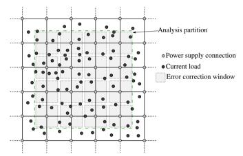
**Fig. 16.** Partition of a resistive flip-chip power grid with supply connections and load circuits denoted, respectively, with light and dark dots. The error correction windows are shown with small gray boxes around each supply connection node. (For interpretation of the references to color in this figure legend, the reader is referred to the web version of this article.)
