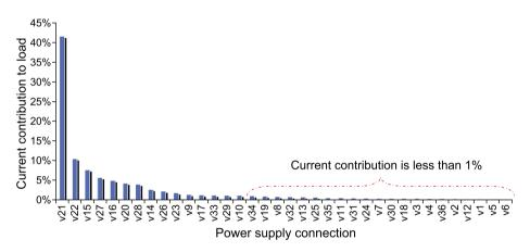
**Fig. 13.** Percent current provided to the current load  $L_2$  placed within a uniform power grid via the power supply connections, as illustrated in Fig. 11. Note that more than 40% of the current is provided by the closest power supply connection,  $V_{21}$ . The current contribution of a supply connection is significantly smaller with distance.
