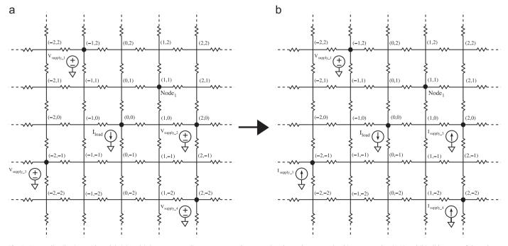
**Fig. 7.** Power distribution grid model: (a) multiple power supplies are connected to several nodes and a current load is connected at (0,0) and (b) all but one of the voltage sources are replaced with an equivalent current source.
