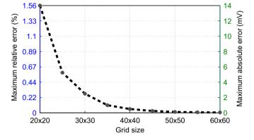
**Fig. 14.** Maximum error for different grid size assuming a model of a finite power grid with an infinite mesh structure. The percent relative error as compared to SPICE and the absolute error are shown, respectively, on the left and right axes. Note that the error decreases significantly with increasing grid size.
