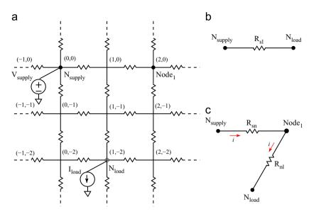
**Fig. 3.** Power distribution grid model: (a) one power supply connected at (0,0) and one current load connected at (1,-2), (b) corresponding reduced effective resistance model between the power supply and the load, and (c) the effective resistance model to determine the voltage at an arbitrary node Node<sub>1</sub> within the power grid.
