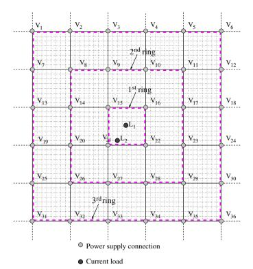
**Fig. 11.** A portion of a typical power grid with C4 bumps illustrated with light dots and load devices with dark dots. Most of the current sunk by the load devices,  $L_1$  and  $L_2$ , is provided by the supply connections forming the first ring. Power supply connections within the third ring contribute less than 1% of the total current to these load devices.
