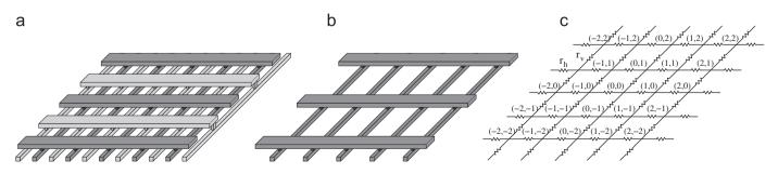
Fig. 1. Two layer orthogonal metal lines connected with vias; (a) two layer power and ground distribution networks where the power and ground lines are illustrated, respectively, with dark and light grey, (b) a two layer power distribution network, and (c) a resistive mesh model of the power distribution network.
