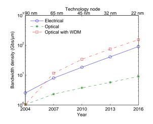
Fig. 5. Bandwidth density of electrical and optical interconnects.
