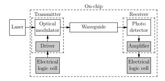
Fig. 2. An on-chip optical interconnect data path.
