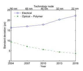
Fig. 3. Comparison of standard deviation of electrical and optical interconnect delays.
