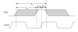
Fig. 4. Timing diagram of data and clock waveforms.
