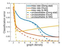
Figure 2: Label propagation for the problem "1" vs. "2" of MNIST with different class size proportions: 1 to 4 (left), 1 to 1 (middle) or 4 to 1 (right). Missclassification rate for different number of edges per node.
