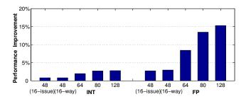
**Figure 2.** Average performance improvement for SPEC Int and SPEC FP applications as a result of increasing issue width, entire processor pipeline width, or the LQ size.
