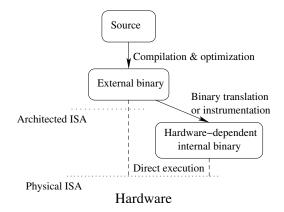
**Figure 1.** Instruction set architecture support for low-level software-hardware cooperative optimization.
