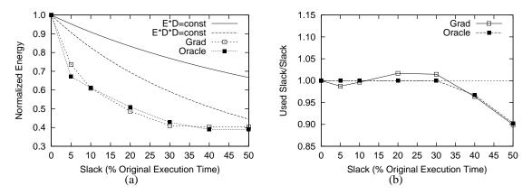
Figure 9: Effect of exploiting different execution slacks: resulting energy consumed by the applications (a) and fraction of the slack that is used up (b).
