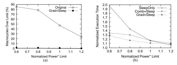
Figure 8: Impact of enforcing different  $Power^*$  limits in the chip: fraction of thermal macrocycles over the  $Power^*$  limit (a) and resulting execution time of the applications (b).
