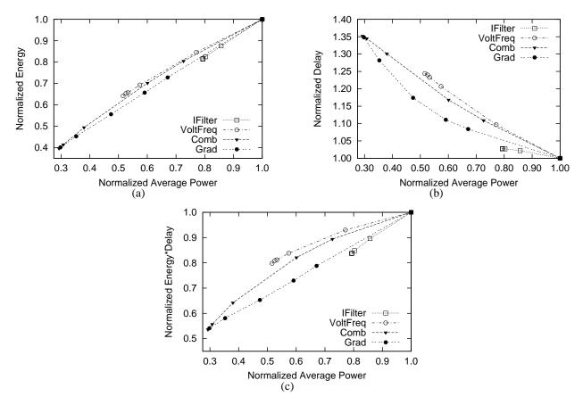
Figure 6: Impact of dynamically applying a combination of energy-management techniques: total energy consumed by the applications (a), their execution time (b), and their energy-delay product (c). The data is organized as in Figure 5.
