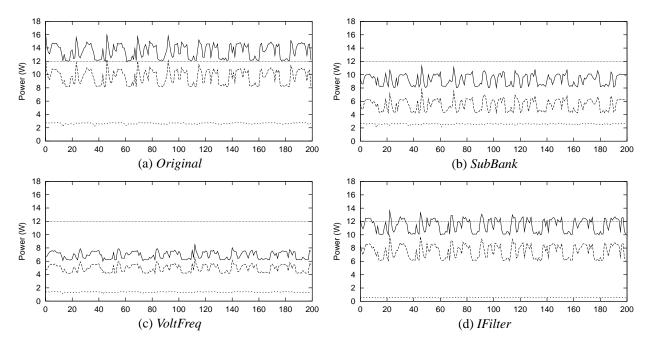
Figure 4: Power dissipated in a section of *BSOM* for different environments. The unit in the X-axes is 1,000 cycles or  $1.25 \mu s$ .
