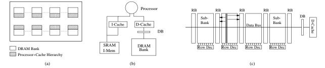
Figure 3: Chip architecture modeled: overview of the chip (a), per-processor memory hierarchy (b), and per-processor DRAM bank organization (c). In the charts, *RB*, *DB*, and *Row Dec* stand for row buffer, data buffer, and row decoder, respectively.
