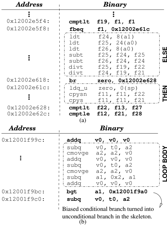
Figure 3. Examples of empty if-then-else block (a) and loop (b) in the skeleton of real applications. Instructions selected in the skeleton are shown in bold.
