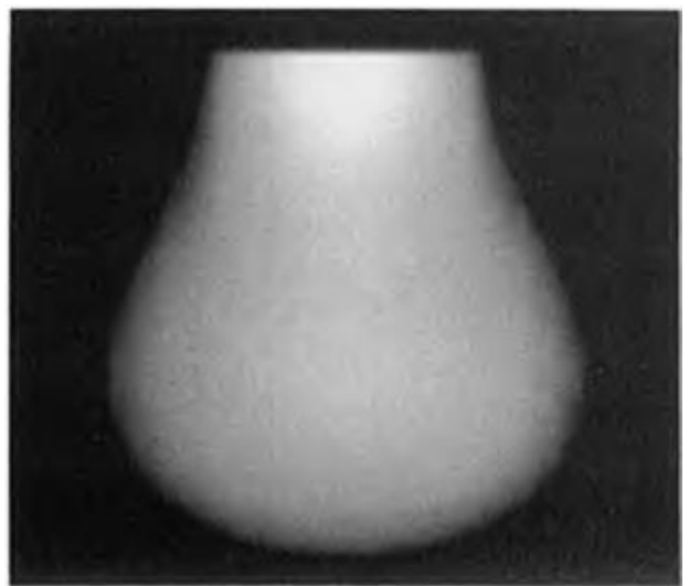
FIG. 13. Liver scan simulation using our theory for a homogeneous, bounded medium with a Gaussian vibration source.
