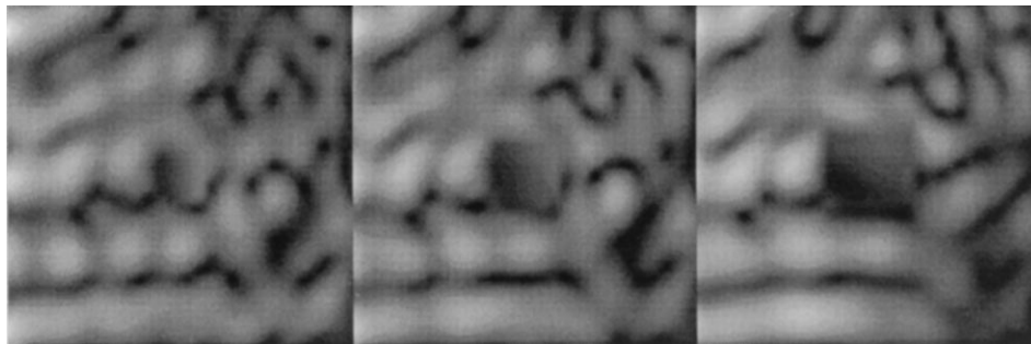
Fig. 9. Grey-scale images of the vertical displacement amplitudes at a vibration frequency 400 Hz for different size lesions where E/E_0 = 5 : left = 4 mm \times 4 mm; middle = 6 mm \times 6 mm; right = 8 mm \times 8 mm.
