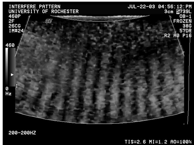
**Figure 4.** Sonoelastography image of shear wave interference pattern on GE Logiq 700. The medium is 5% gelatin phantom. Both sources vibrate at 200 Hz. The peak vibration amplitude in the direction of the ultrasound wave is mapped to a grey scale.
