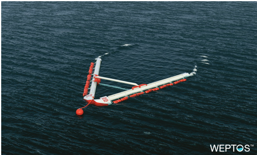
Fig. 1 The WEPTOS WEC model in testing. Thomsen, Kirt. WEPTOS, Pecher, Arthur, Jens P. Kofoed, Tommy Larsen, and Tanguy Marchalot N.d. Web.
