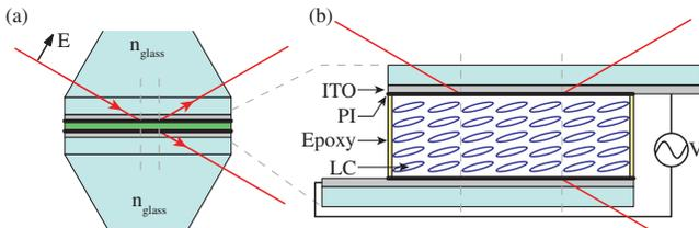
FIG. 1 (color online). Diagram of the double-prism system. In (a) a liquid crystal cell is sandwiched between two glass equilateral prisms. An exploded diagram of the liquid crystal cell is shown in (b), with the liquid crystal (LC), indium tin oxide (ITO) layer and polyimide alignment (PI) layer labeled.
