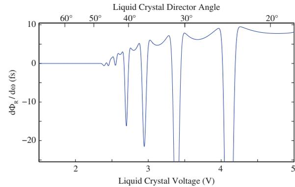
FIG. 4 (color online). Predicted  $\partial\Phi_R/\partial\omega$  based on the  $4 \times 4$  matrix method described in the text for 727-nm light propagating through an 8-micron liquid crystal cell. The parameters used are  $\theta = 63.5^\circ$ ,  $n_{\text{glass}} = 1.77$ ,  $n_e = 1.63$ , and  $n_o = 1.54$ .
