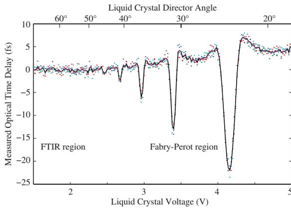
FIG. 3 (color online). Reflection delay in FTIR from a double-prism barrier system. The black line is the arithmetic mean of four individual data sets, shown in colored dots. Each data point represents an individual Hong-Ou-Mandel trace with 102 seconds of integration time.
