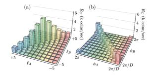
FIG. 2. (Color online) Coincidence count rates for the OAM basis (a) and the angle basis (b) for the case of D=11. For this data set, there is no neutral density filter placed between the pump and the BBO crystal. The integration time for each measurement point is 1 s.
