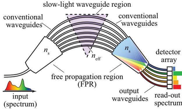
Fig. 1. Schematic diagram of a slow-light arrayed-waveguide-grating spectrometer.
