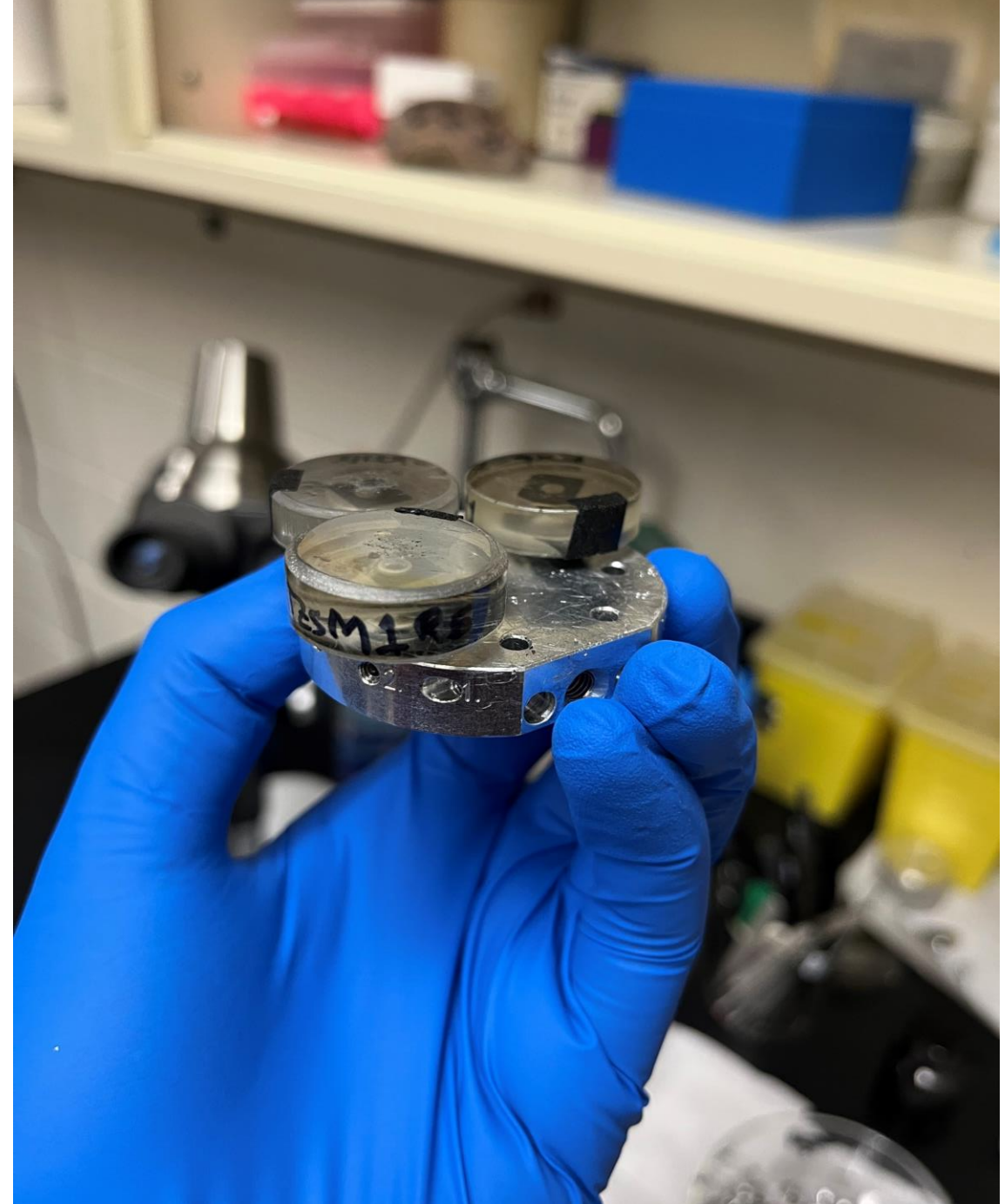
Fig.1 : Carbon – coated epoxy mounts on sample holder of the SEM
