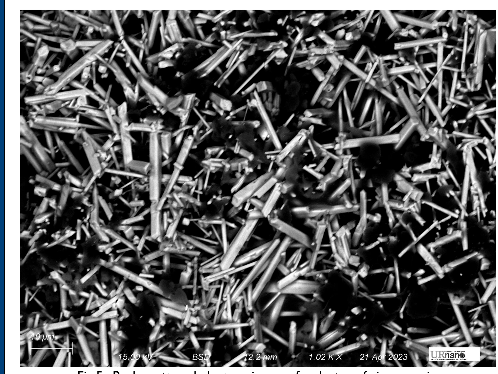
Fig.5 : Back-scattered electron image of a cluster of zircon grains
