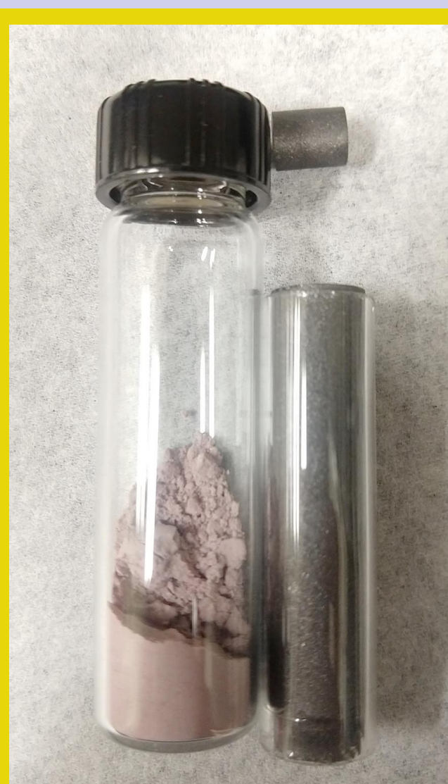
Fig. 2. The lab-created Sudbury sample (left) with the graphite furnace (right), part of the apparatus that entered into the piston cylinder.
