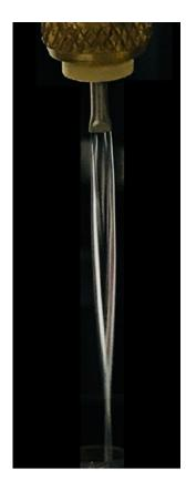
Fig. 10 Photo of a  $120 \mu m$  thick water film formed by a water jet with a flat nozzle [62]. The laser beam is focused into the center of the film where is flat and stable
