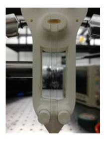
**Fig. 2** Photo of the water film. Two aluminum wires are separated by 4 mm. The thickness of the water film is controlled by the water flow rate
