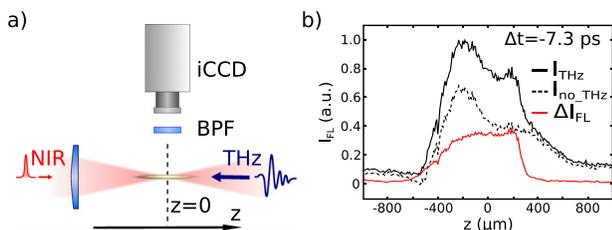
FIG. 4. (a) Experimental setup for taking the fluorescence images. The NIR (red) and THz (blue) pulses travel in opposite directions. The plasma is imaged from the side with an iCCD camera through a narrowband filter (BPF) centered at 337 nm. (b) Plasma fluorescence cross-sections with (black) and without (dashed, black) THz illumination. The red curve is the spatially resolved fluorescence enhancement calculated by subtracting the fluorescence profile with and without THz illumination.
