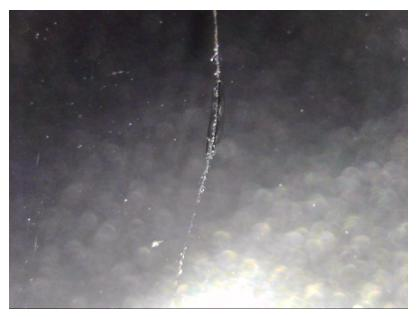
**Picture 5:** Picture of lens under darkfield lighting with source at 60 degrees from the ground. The light from the source can be seen at the bottom of the picture.
