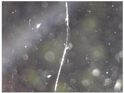
**Picture 1:** x20 mag picture of lens under Darkfield at 0 degrees. Ambient lighting still present.
