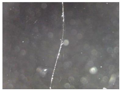
**Picture 4:** Picture of lens under darkfield lighting with source angled at 30 degrees above the ground. Less contrast of small features.
