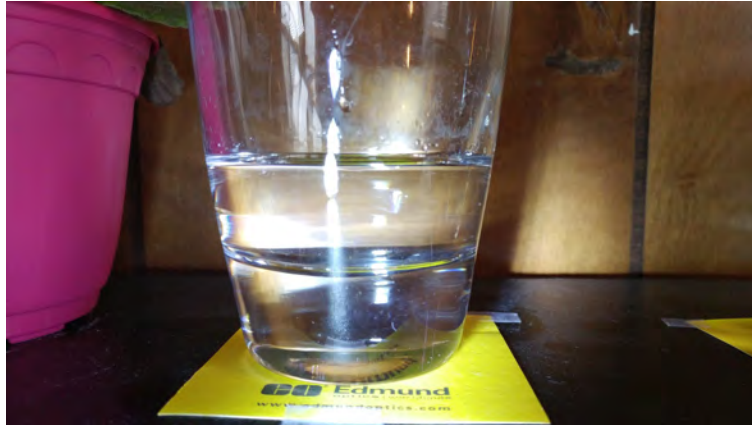
Figure 6: Front lighting Calcium Fluoride in Ethylene Glycol
