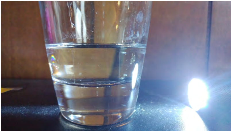
Figure 5: Side lighting Calcium Fluoride in Ethylene Glycol
