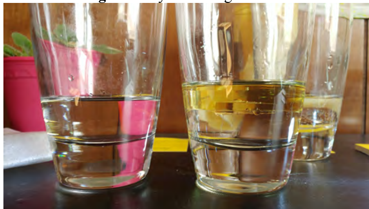
Figure 8: Calcium Fluoride in Ethylene Glycol and Ethylene Glycol with Oil
