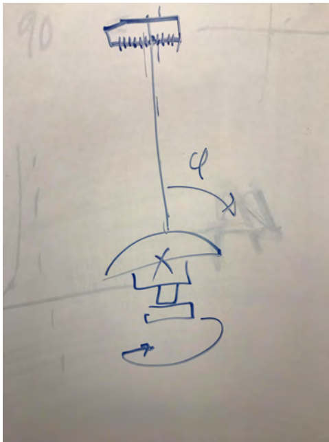
Figure 1: Rough white-board sketch (left) and computer block diagram (right) of potential testing set-up including the lens being tested and a bar target. Data will be recorded at a number of polar (lens) and azimuth (bar target) angle combinations.
