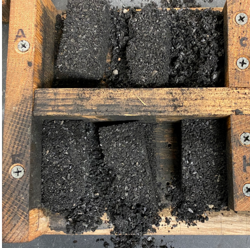
Figure 4: Biochar (75%), Plastic (20%), and Sand (5%) Prototype Bricks
