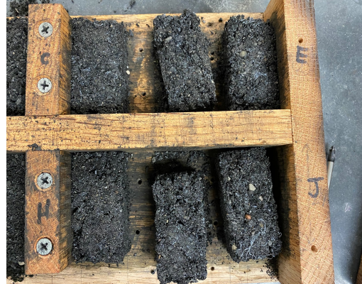
Figure 5: Biochar (50%), Plastic (40%), and Sand (10%) Prototype Bricks
