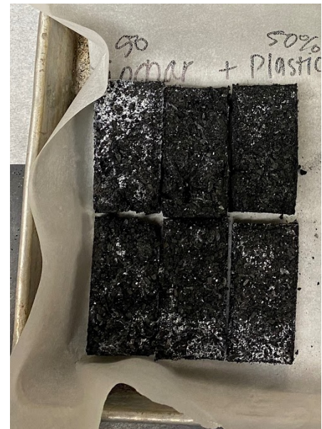
Figure 7: Biochar (50%) and Plastic (50%) Prototype Bricks
