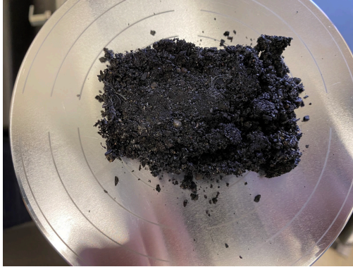
Figure 23: 50% Biochar, 40% Plastic, & 10% Sand Prototype Brick after Maximum Load
