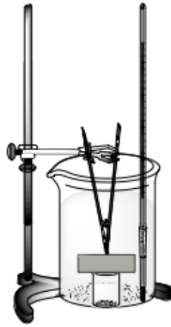
Figure 10: Water Absorption Set-up with Biochar Brick
