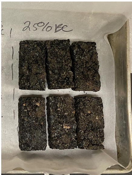
Figure 6: Biochar (25%), Plastic (60%), and Sand (15%) Prototype Bricks
