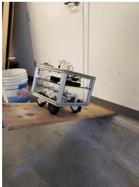
Figure 13. This figure shows the setups for physical tilting test.
